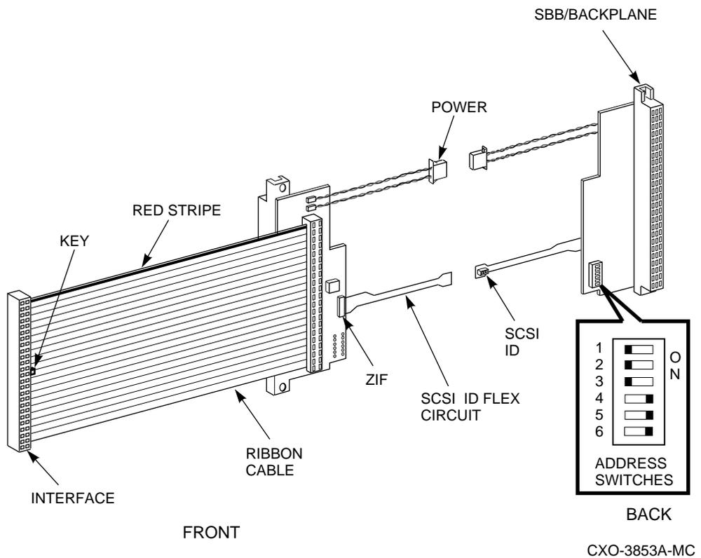
**Figure 10 RRD42 Device Interface Connection**
