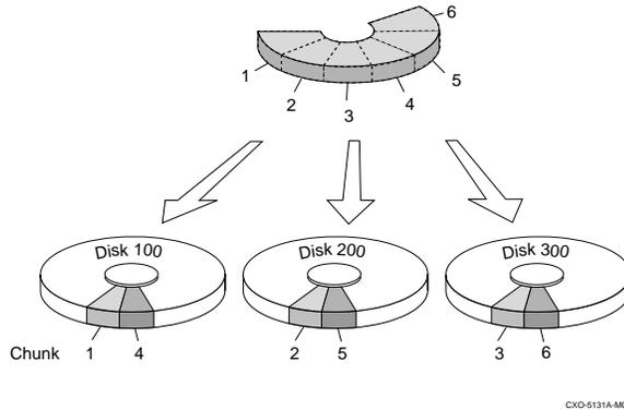
The relationship between the chunk size and the average request size determines if striping maximizes the request rate or the data-transfer rate. You can set the chunk size or let the controller set it automatically. See *Chunk size* on page 3-18 for information about setting the chunk size.
