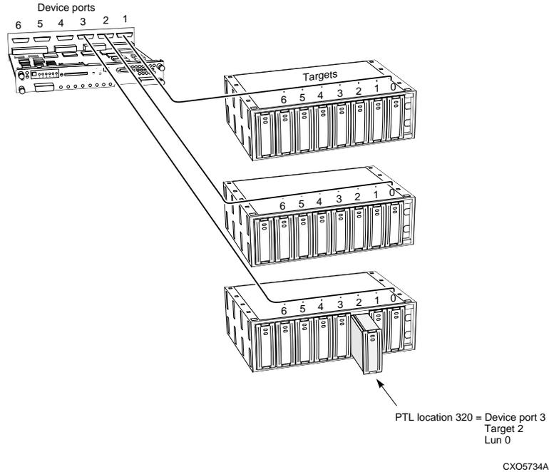
The controller uses the PTL location to name each device that you add to your subsystem with the CONFIG utility or CFMENU. (Factory-installed devices are added with the CONFIG utility. Thus, their names derive from their PTL locations.) For example, if the controller finds a disk in PTL 320, it names it DISK320; if it finds a tape drive at PTL 320, it names it TAPE320.
