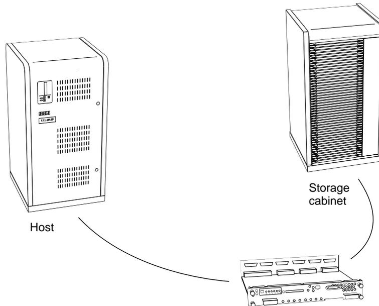
From the subsystem's perspective, the controller receives the I/O requests from the host and directs them to the devices in the subsystem. Since the controller processes all of the I/O requests, it eliminates the host-based processing that's typically associated with reading and writing data to multiple storage devices.
