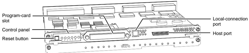
Under normal circumstances, you won't need to remove the controller from its cabinet. For this reason, the components that you'll use most often are conveniently located on the front panel. For example, the local-connection port provides a convenient way to connect a terminal to your controller so that you can configure it for the first time.
