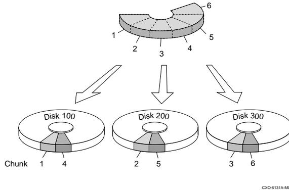
The relationship between the chunk size and the average request size determines if striping maximizes the request rate or the data-transfer rate. You can set the chunk size or let the controller set it automatically. See *Chunk size* on page 3-19 for information about setting the chunk size.
