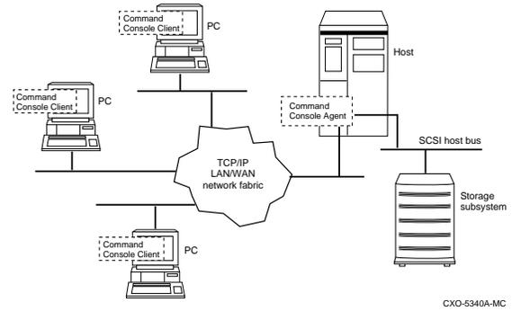
Agent acts as Client's assistant in controlling your storage subsystem. Commands sent from Client are received by Agent and are routed to the storage subsystem via the subsystem's SCSI host bus. Subsystem status is transmitted back to Client from Agent via the network connection. Agent can also be used for access protection.
