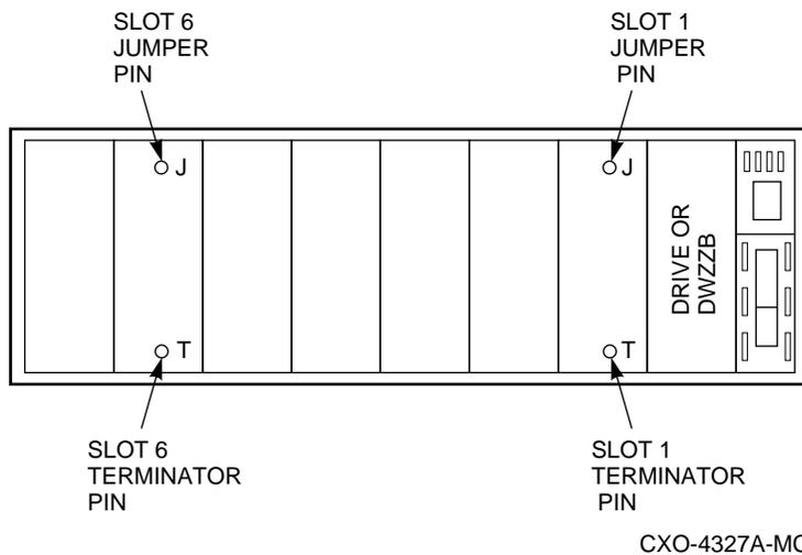
When installed, the terminator or jumper position can be determined from the front of the shelf by removing the SBBs in slot 1 and 6. An indicator pin protruding through the backplane in the T position in the bottom of the slot indicates a terminator is installed in that position. An indicator pin protruding through the J position in the top of the slot indicates a jumper is installed in that position.
