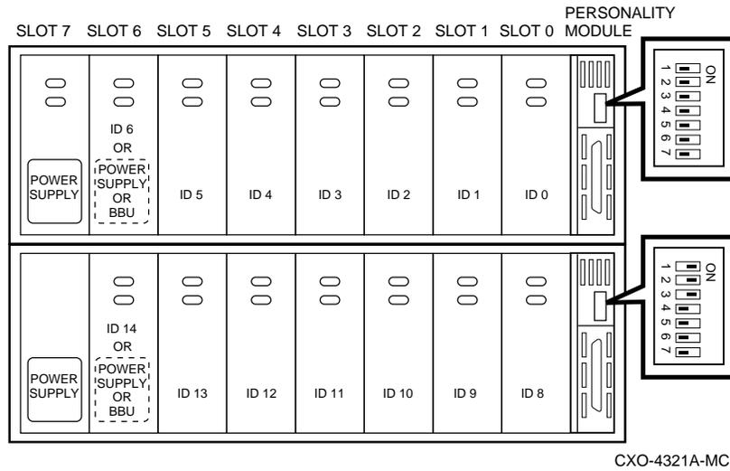
The terminator in the shelf 1 I/O module is automatically disabled if a SCSI cable is connected to the JB1 connector on the front of the module, and is attached to a standard SCSI device at the other end. This daisy chain permits configuration of two shelves with the termination provided in the second shelf.
