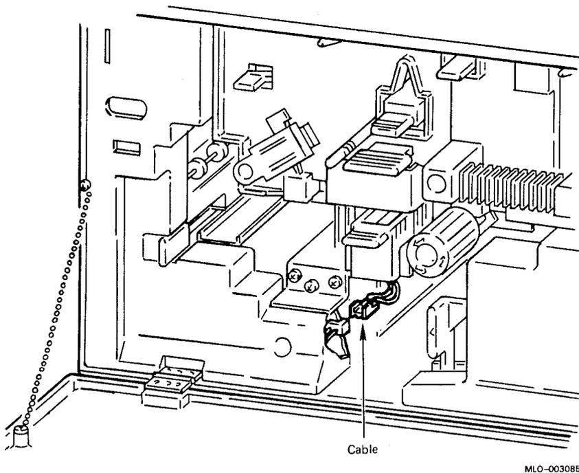
3. Lower the transfer/separation charger guide.
