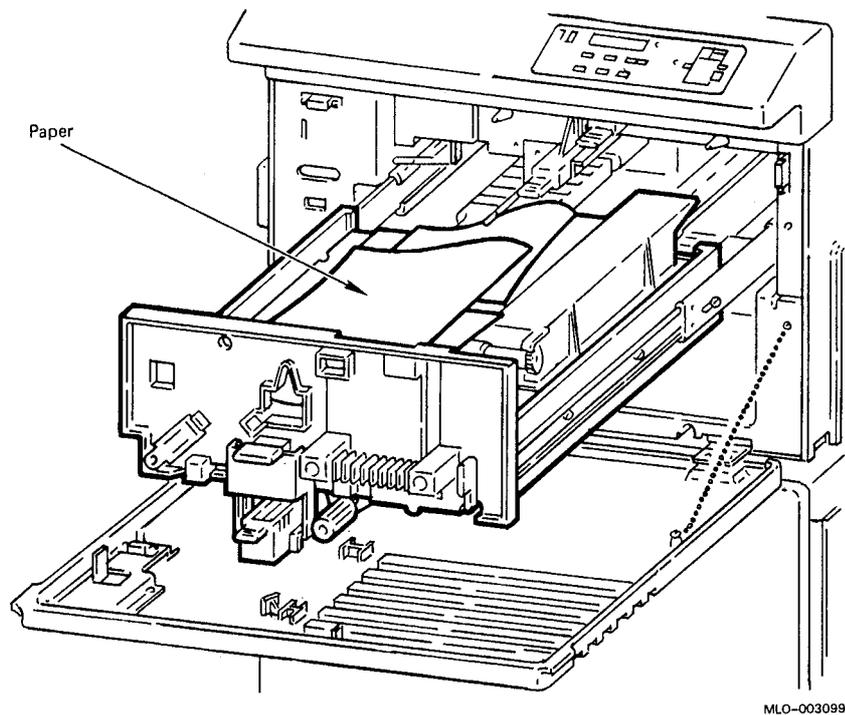
7. Disconnect the development motor cable (CN108) from the mother board.
