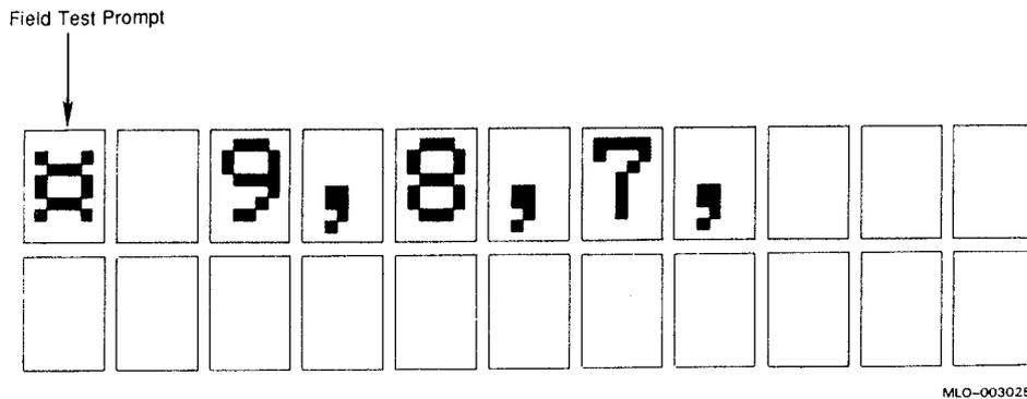
If the self-test finds an error, it displays a self-test error message. If the self-test is successful, the countdown numbers are cleared and you can enter commands.
