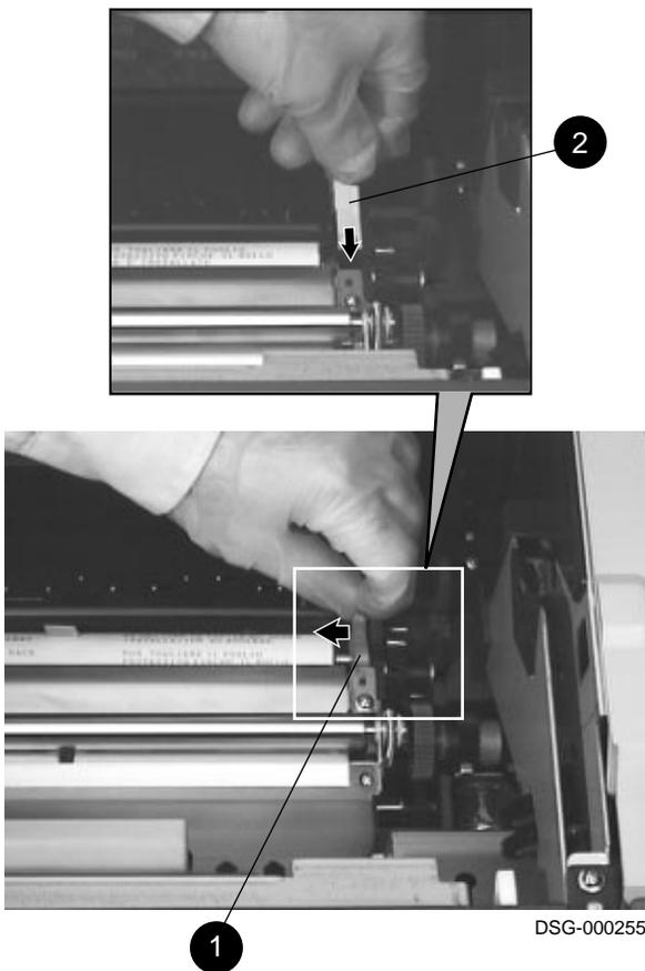
9. Remove the protective covering from the new roller by peeling back the tape and pulling the cover straight up off the roller.
