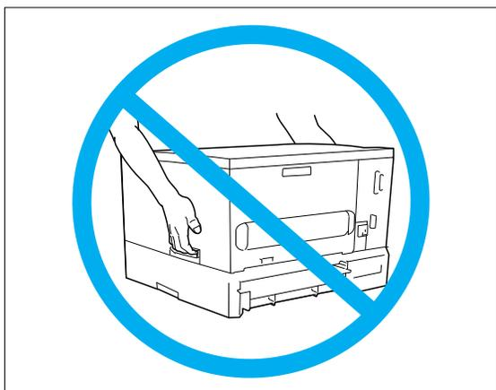
**!** Do not attempt to lift and carry the printer by yourself after installing the Paper Deck.
