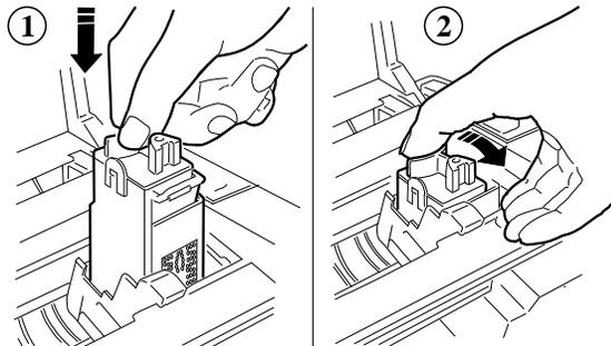
*Inserting and blocking the print head*
