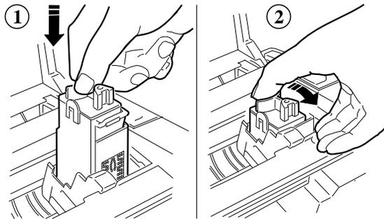
*Inserting and blocking the print head*
