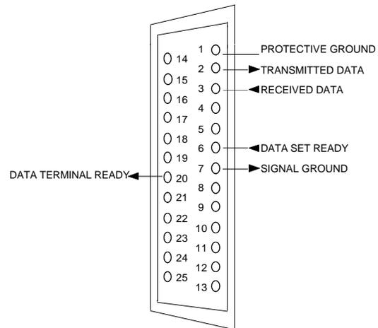
*Serial connector pin positions and corresponding signals*
