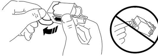
*Removing the protective tape*
