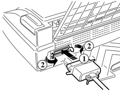
*Inserting the parallel interface cable*
