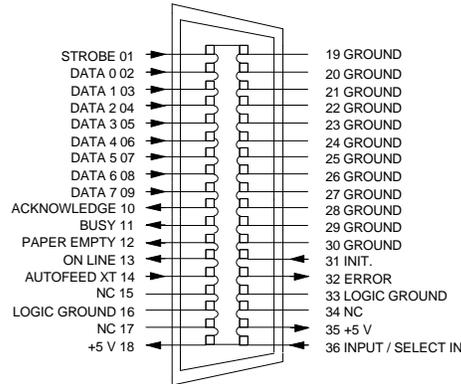
*Connector pins and corresponding signals*
