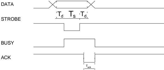
$$\begin{aligned} T_d (min) &= 0.5 \mu s \\ T_s (min) &= 0.5 \mu s \\ T_{ack} &= 5.0 \mu s \end{aligned}$$
