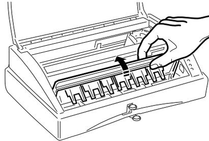
*Removing the paper insertion guide*
