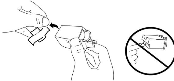
*Removing the protective tape from the ink cartridge*
