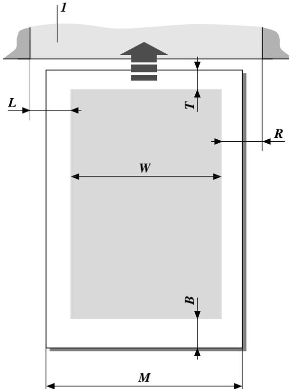
*Dimensions identification (I: Printer mechanical path)*
