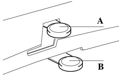
*A: Paper securing lever - B: Paper centering lever*
