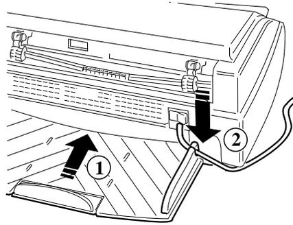
*Inserting the paper input tray*
