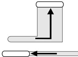
*Moving the levers to secure the paper*
