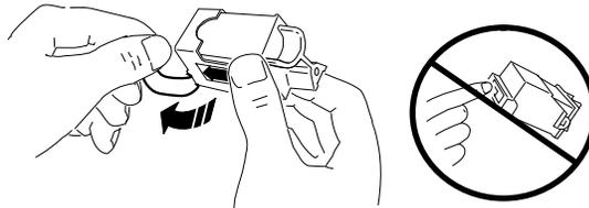
*Removing the protective tape*
