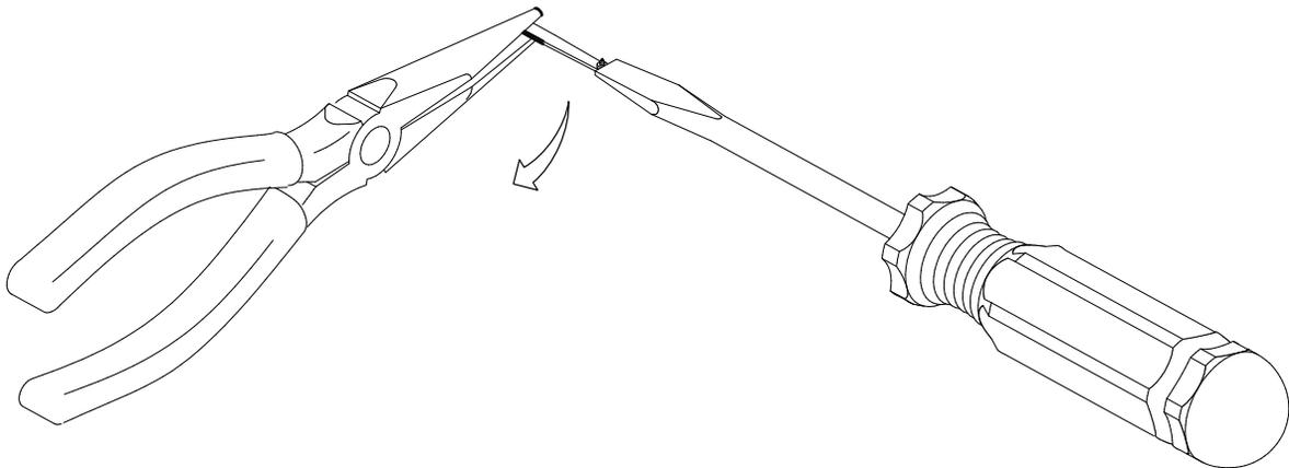
**Figure 5-3. Hammer Spring Retensioning**
