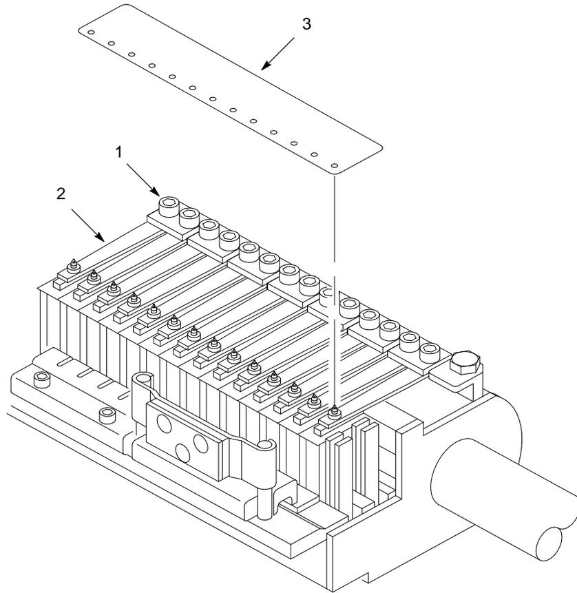
**Figure 5-4. Hammer Tip Alignment**
