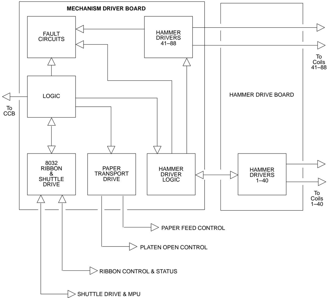
**Figure 2-14. Operational Overview of the Mechanism Driver Board**
