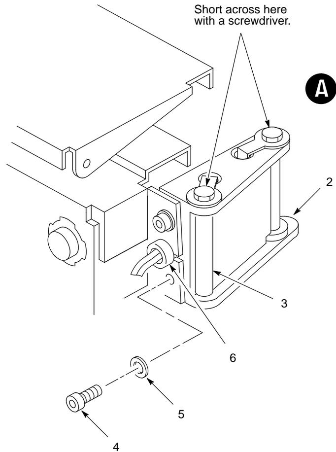
**Figure 5-11. Ribbon Tracking Check and Adjustment**
