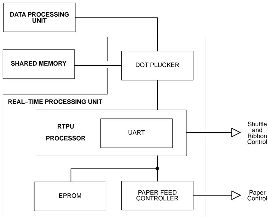
**Figure 2–12. Mechanical Interface Functions of the RTPU**
