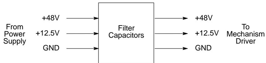
**Figure 2–16. Hammer Driver Power Filtering**
