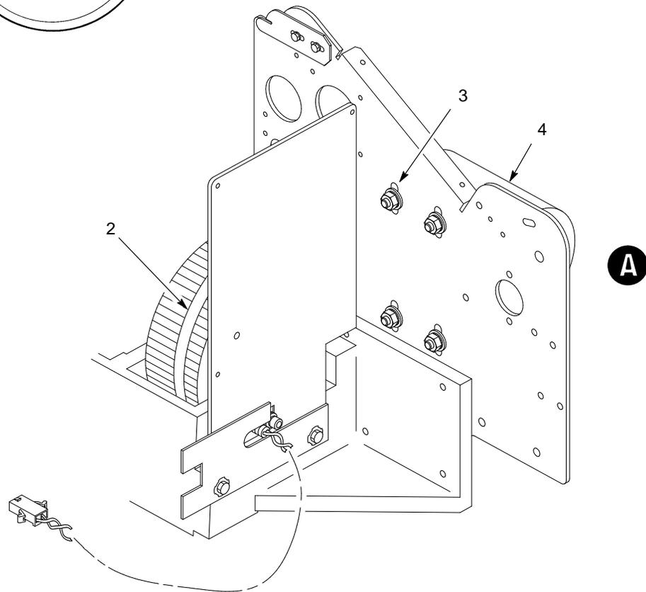
**Figure 5-14. Shuttle Belt Tension Check and Adjustment**
