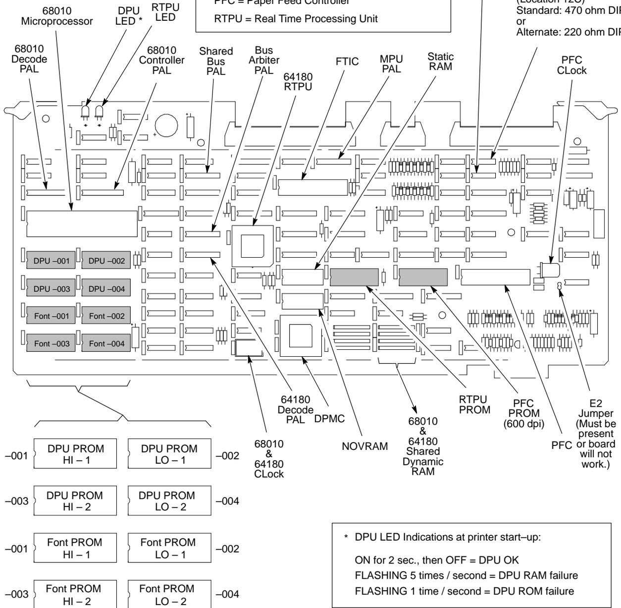
**Figure C-2. Common Controller Board (CCB)**
