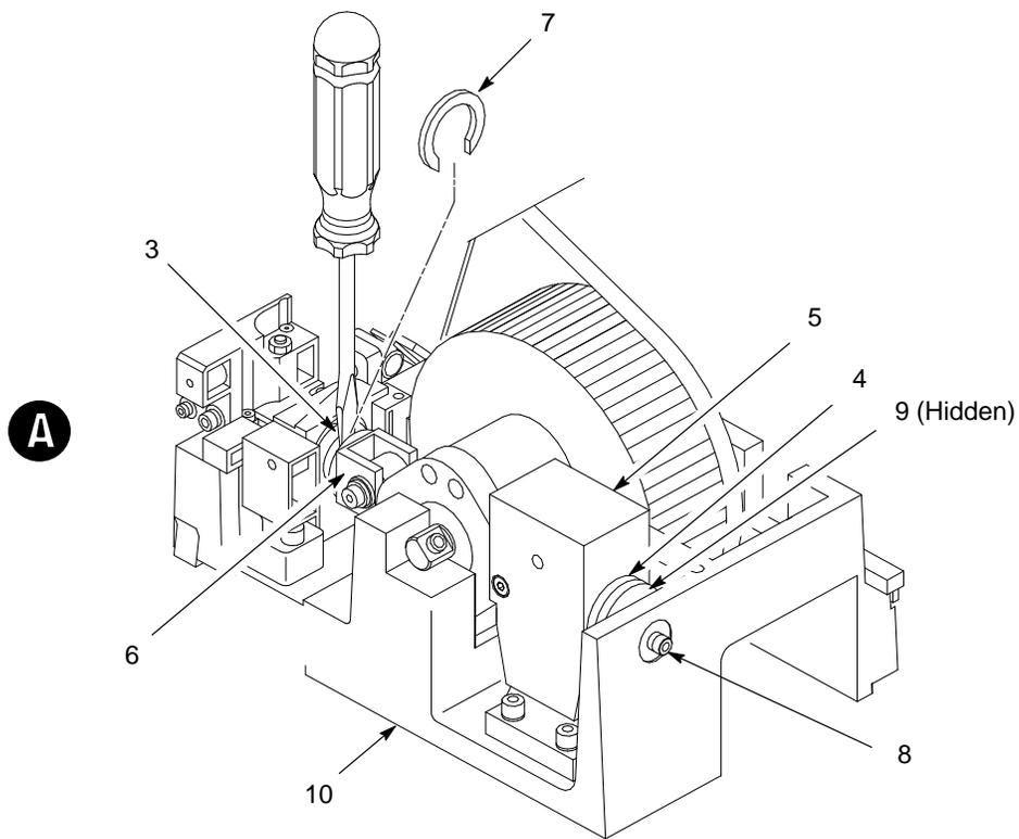
**Figure 5-13. Shuttle Spring Force Adjustment**
