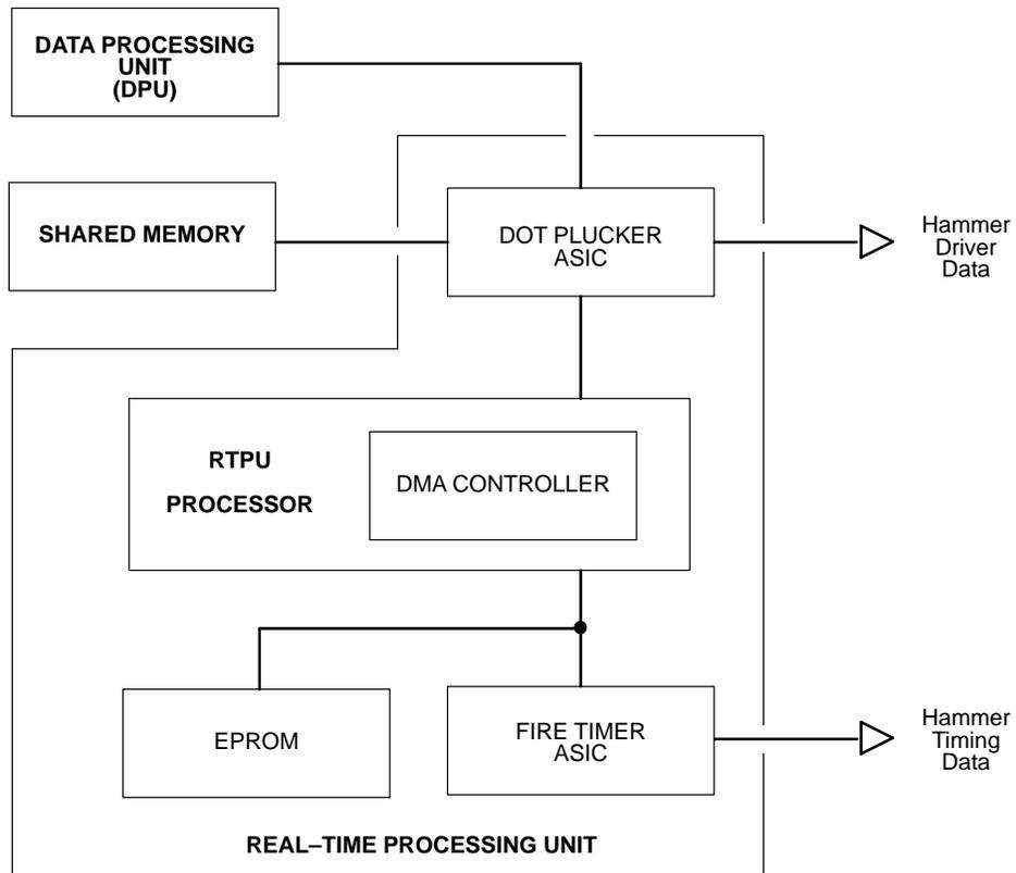
**Figure 2–11. Hammer Driver Interface Functions of the RTPU**
