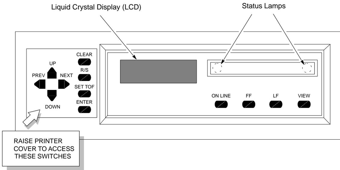
**Figure 1-1. Electrical Controls and Indicators**
