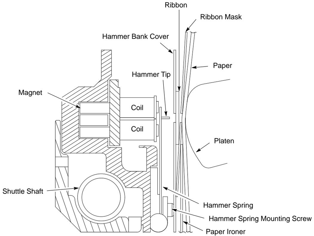
**Figure 2-3. Hammer Spring and Shuttle Arrangement**
