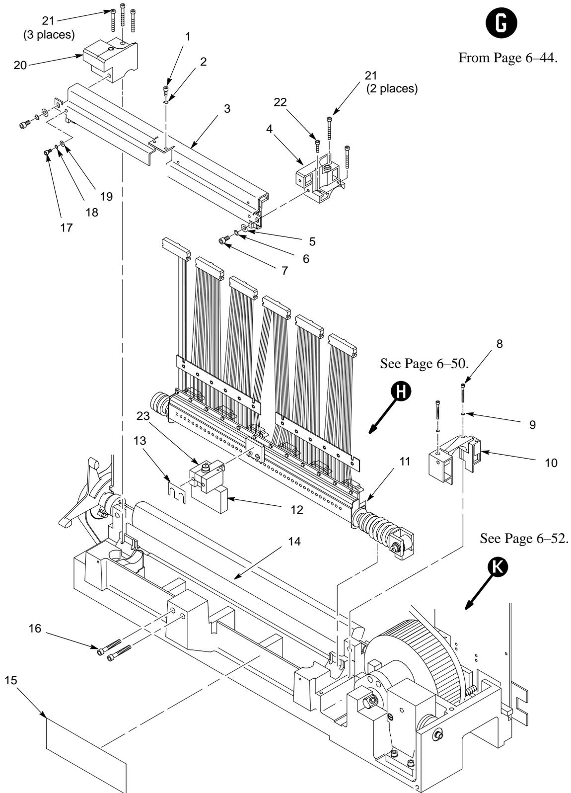
**Figure 6-11. Hammer Bank Assembly**
