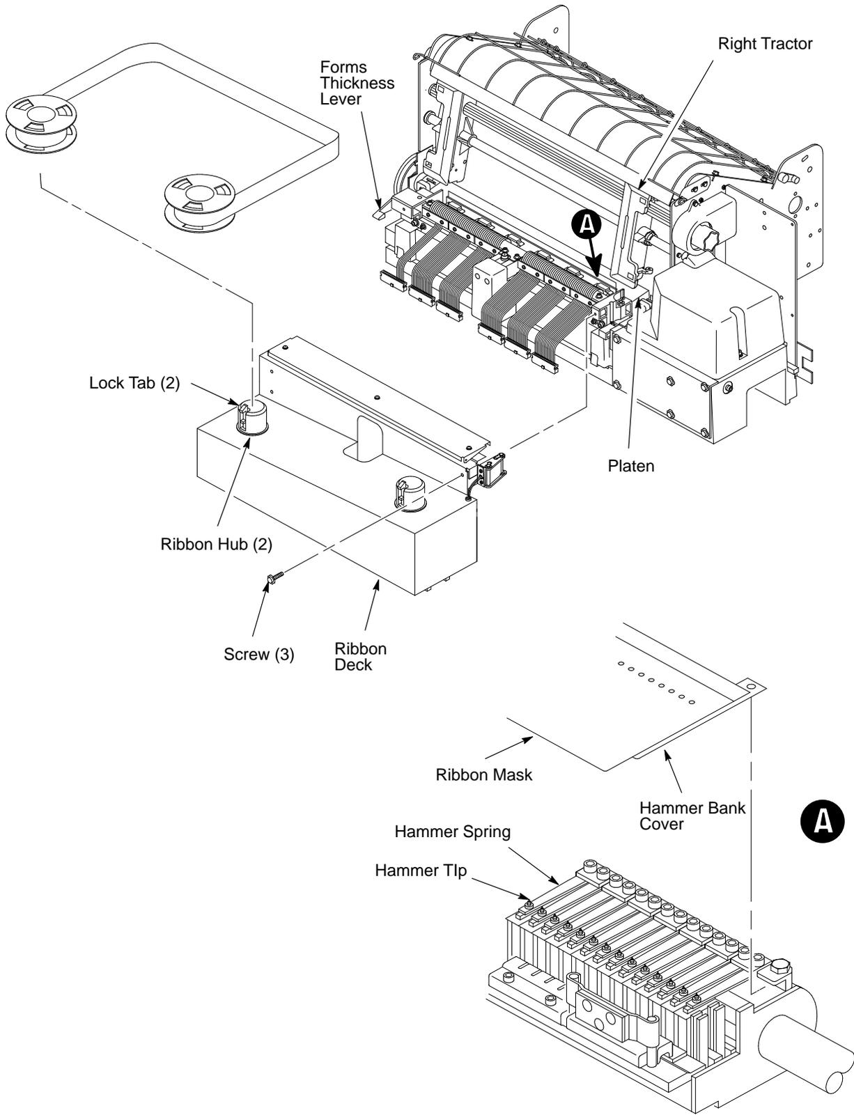
**Figure 3-2. Cleaning Hammer Bank Assembly**
