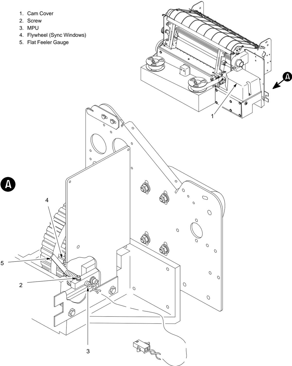
**Figure 5-5. Magnetic Pickup Gap Adjustment**
