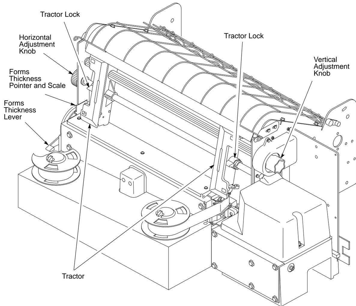
**Figure 1-2. Mechanical Controls**
