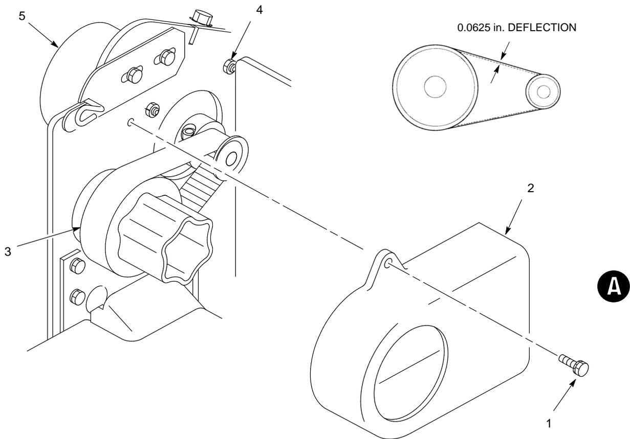
**Figure 5-7. Paper Feed Belt Tension Check and Adjustment**
