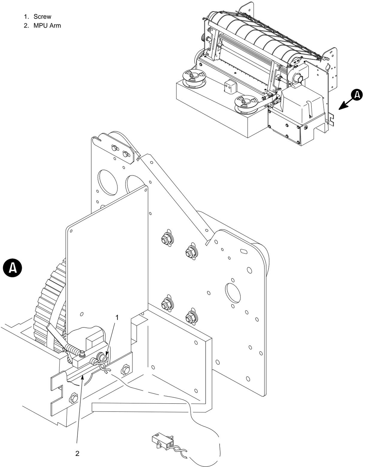
**Figure 5-6. Magnetic Pickup Phasing Adjustment**
