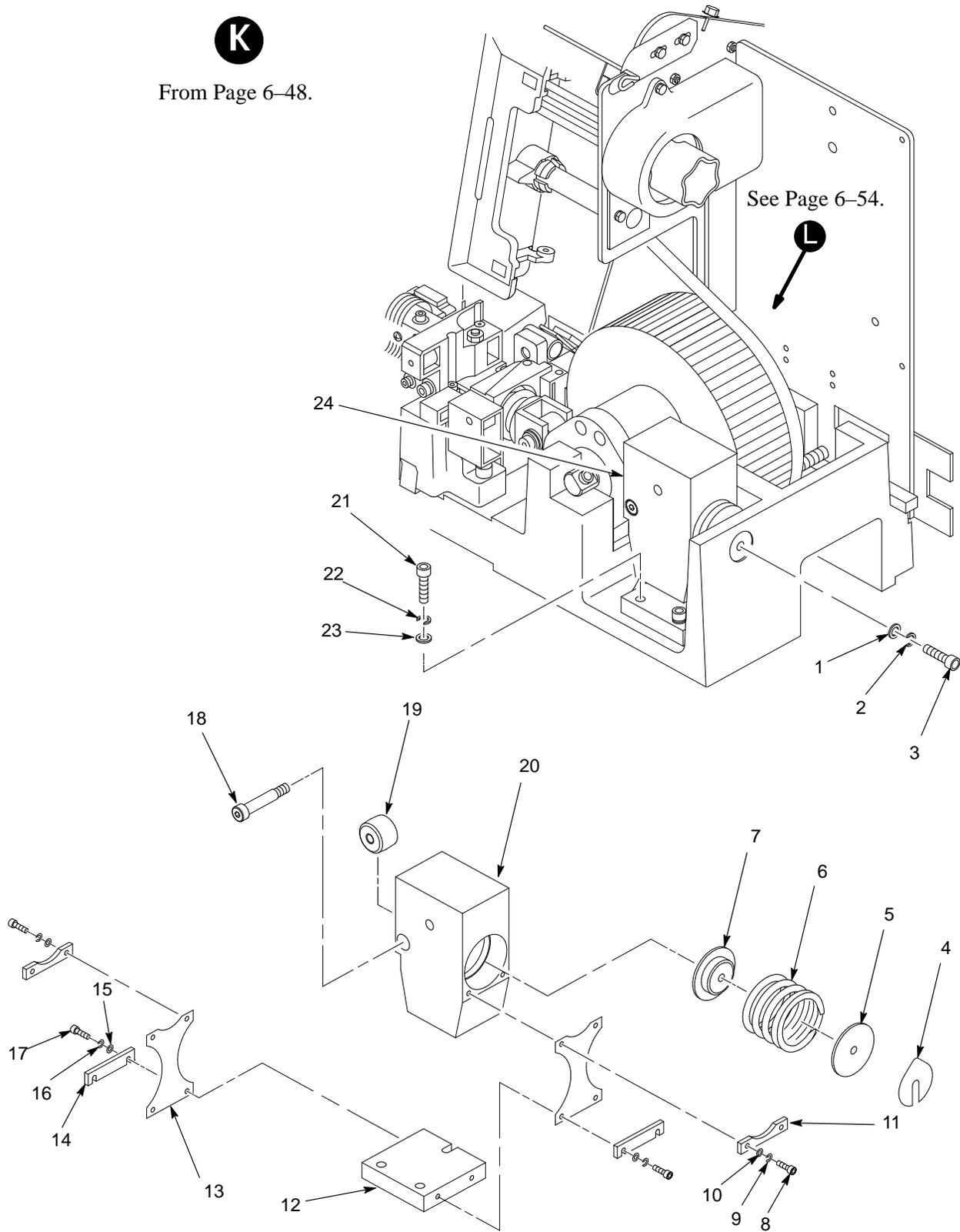
**Figure 6-13. Shuttle Counterweight Assembly**
