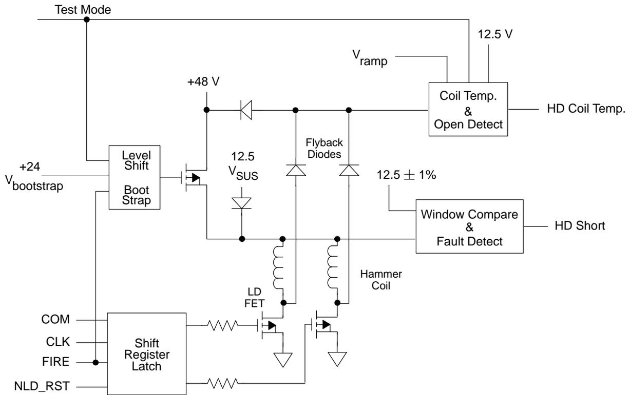
**Figure 2–15. Hammer Driver Logic**
