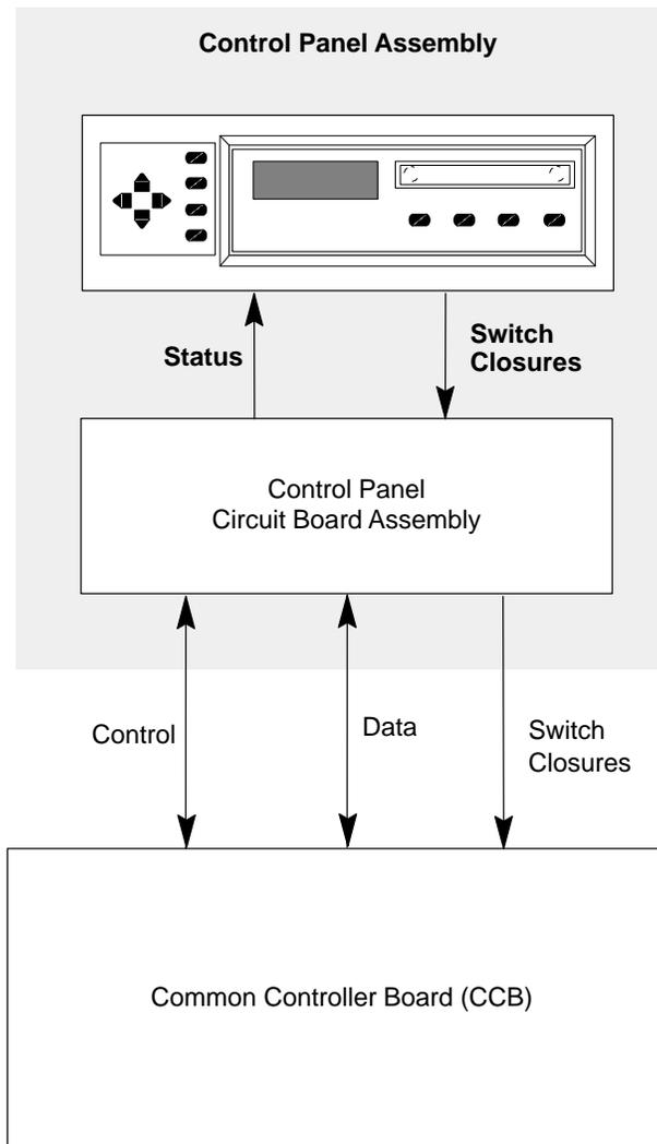
**Figure 2–9. Control Panel Block Diagram**
