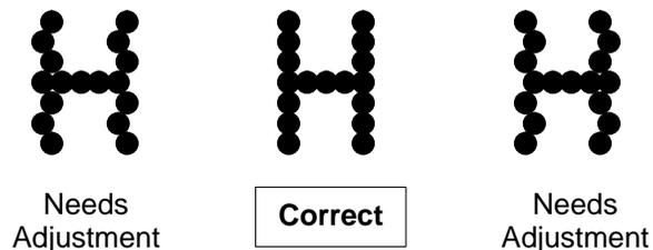
13. When the pattern of H’s is acceptable, press R/S. Printing stops, and the current phase index value is entered into nonvolatile memory.
