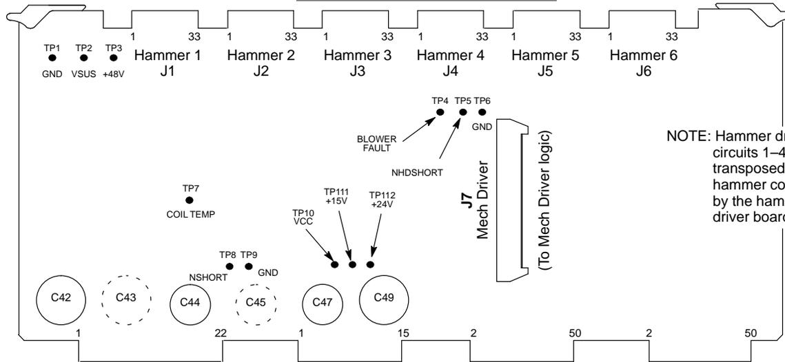
NOTE: Hammer drive circuits 1-48 are transposed to drive hammer coils 41-88 by the hammer driver board.
