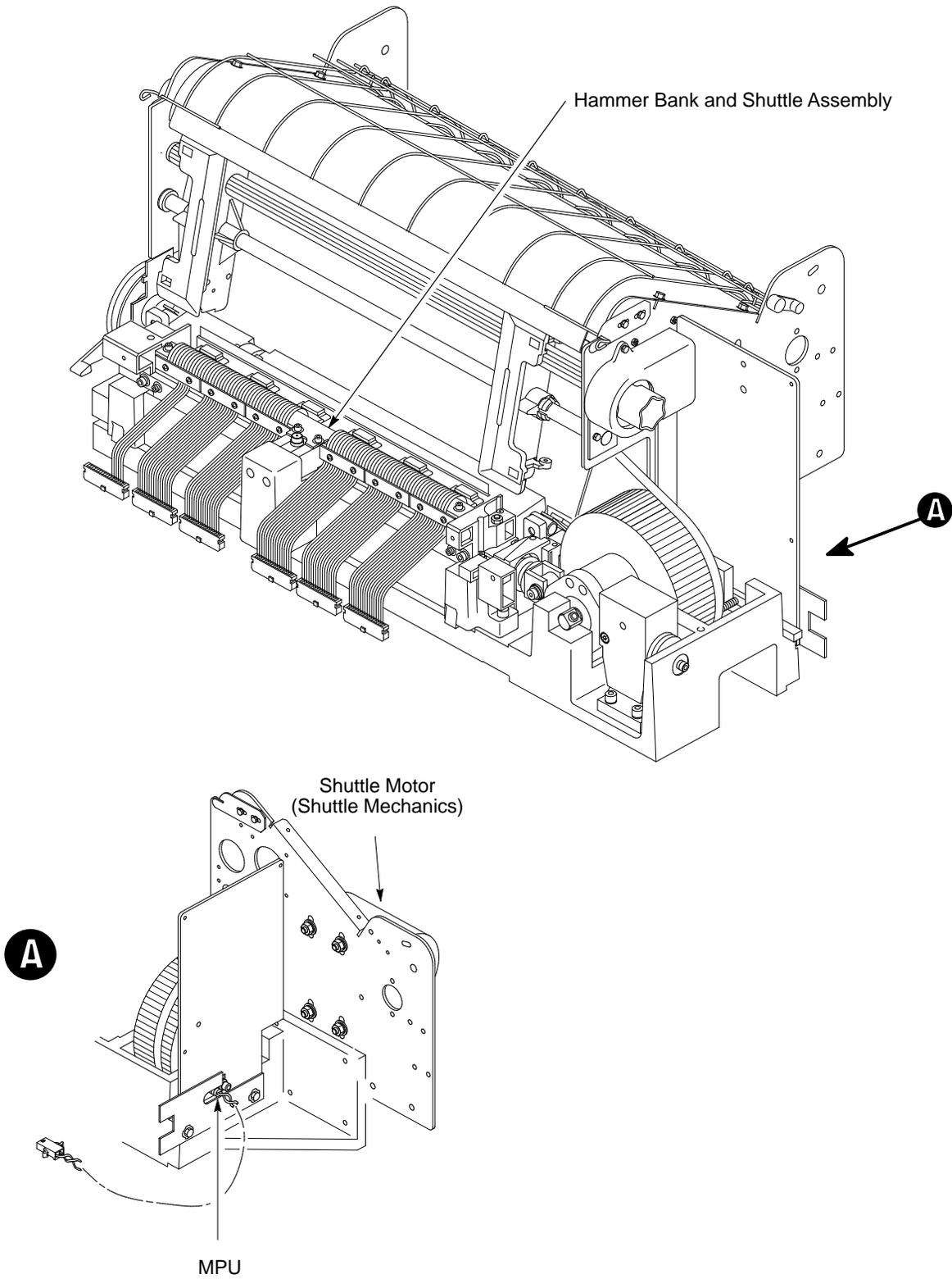
**Figure 2-18. Hammer Bank and Shuttle Mechanical Elements**
