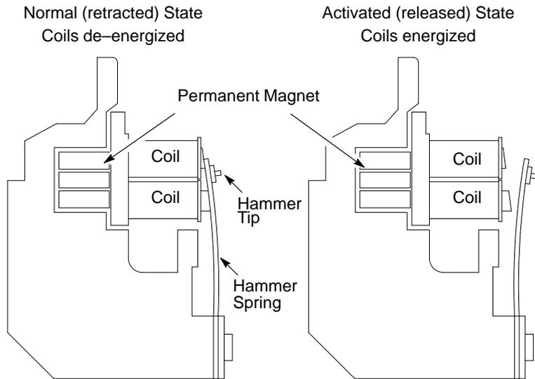
**Figure 2-4. Hammer Spring Action**
