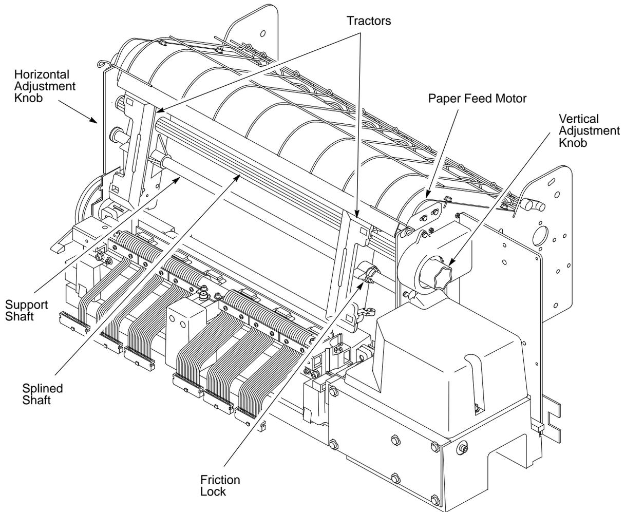
**Figure 2–20. Paper Feed Components**
