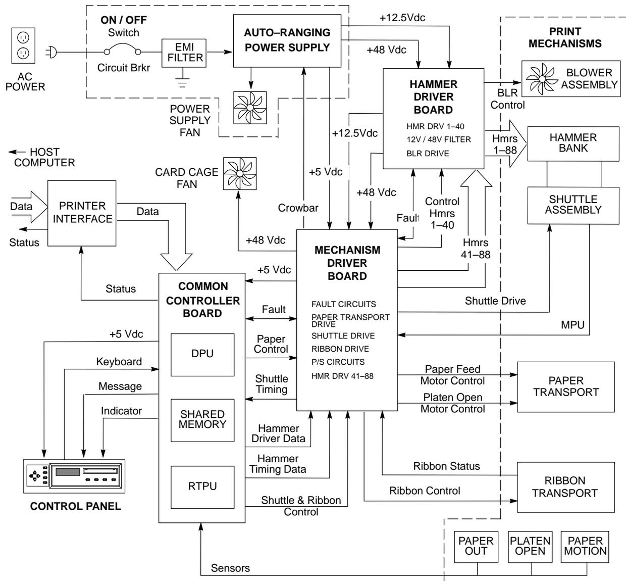
Figure 2-8. Functional Elements of the LG12 Printer
