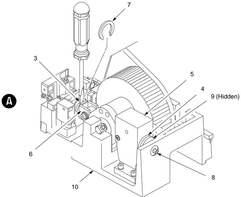
**Figure 5-13. Shuttle Spring Force Adjustment**
