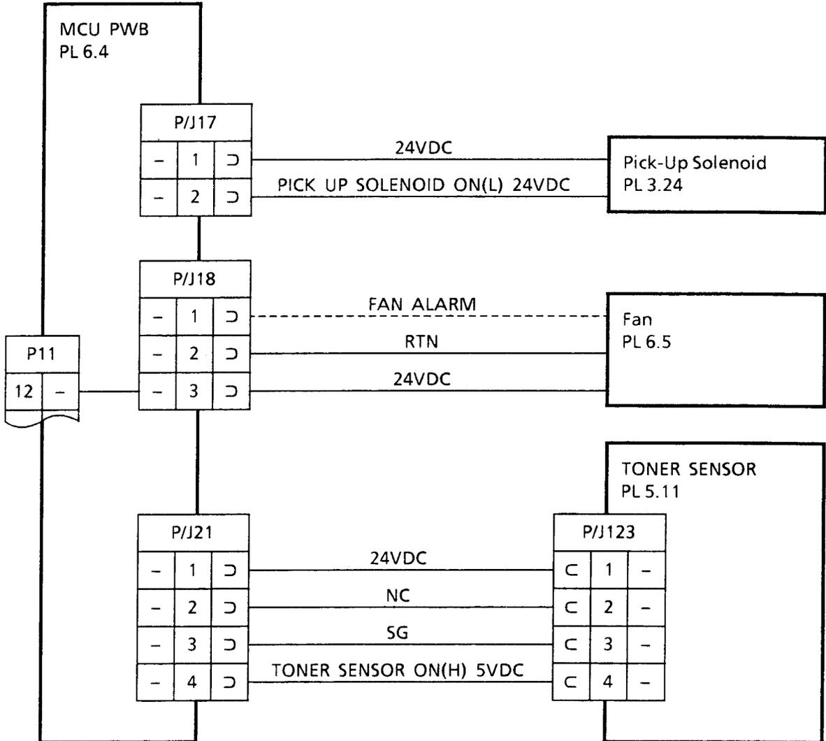
**MCU PWB, Pick-Up Solenoid, Fan, and the Toner Sensor Wiring Diagram**
