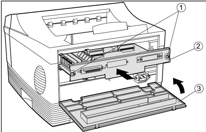
Reinstall and secure the controller (ESS) board and close the rear cover.
