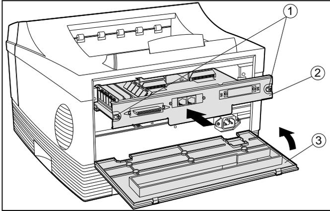
Reinstall and secure the controller (ESS) board thumbscrews and close the rear cover.
