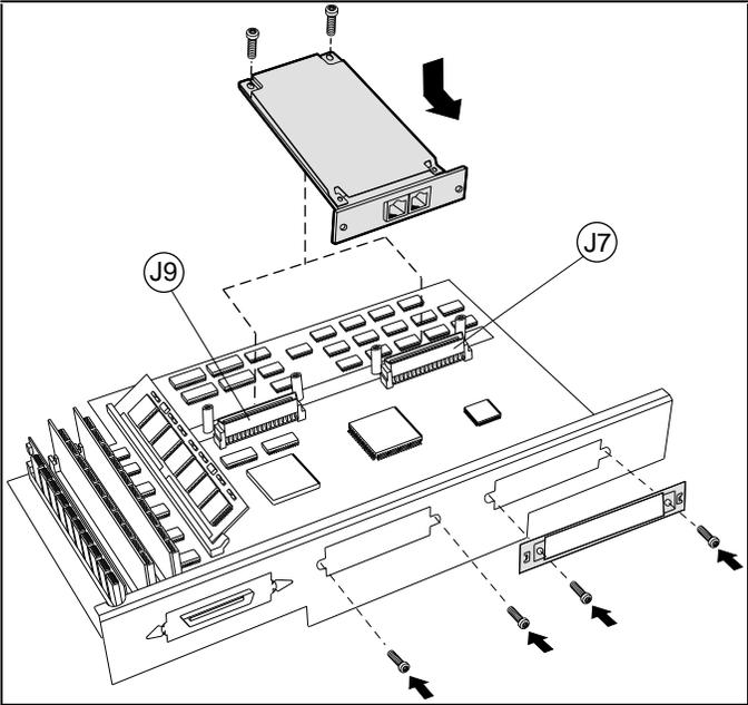
Plug the interface connector into location J7 or J9 and secure.
