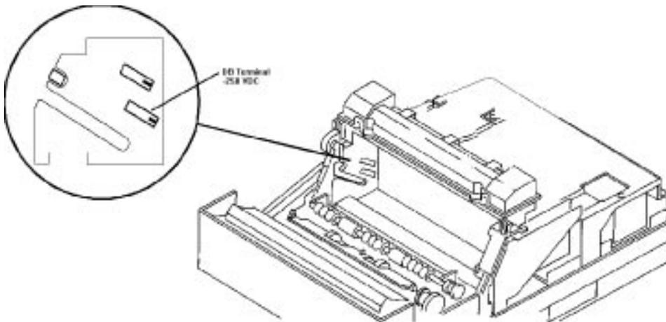
7. Place the black (-) probe of your multimeter on the LVPS frame.
