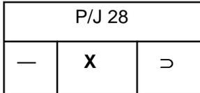
Shows the plug/jack number and the pins. The top line is the plug/jack number.
