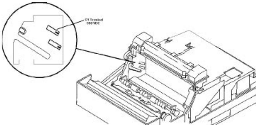
7. Place the black (-) probe of your multimeter on the LVPS frame.
