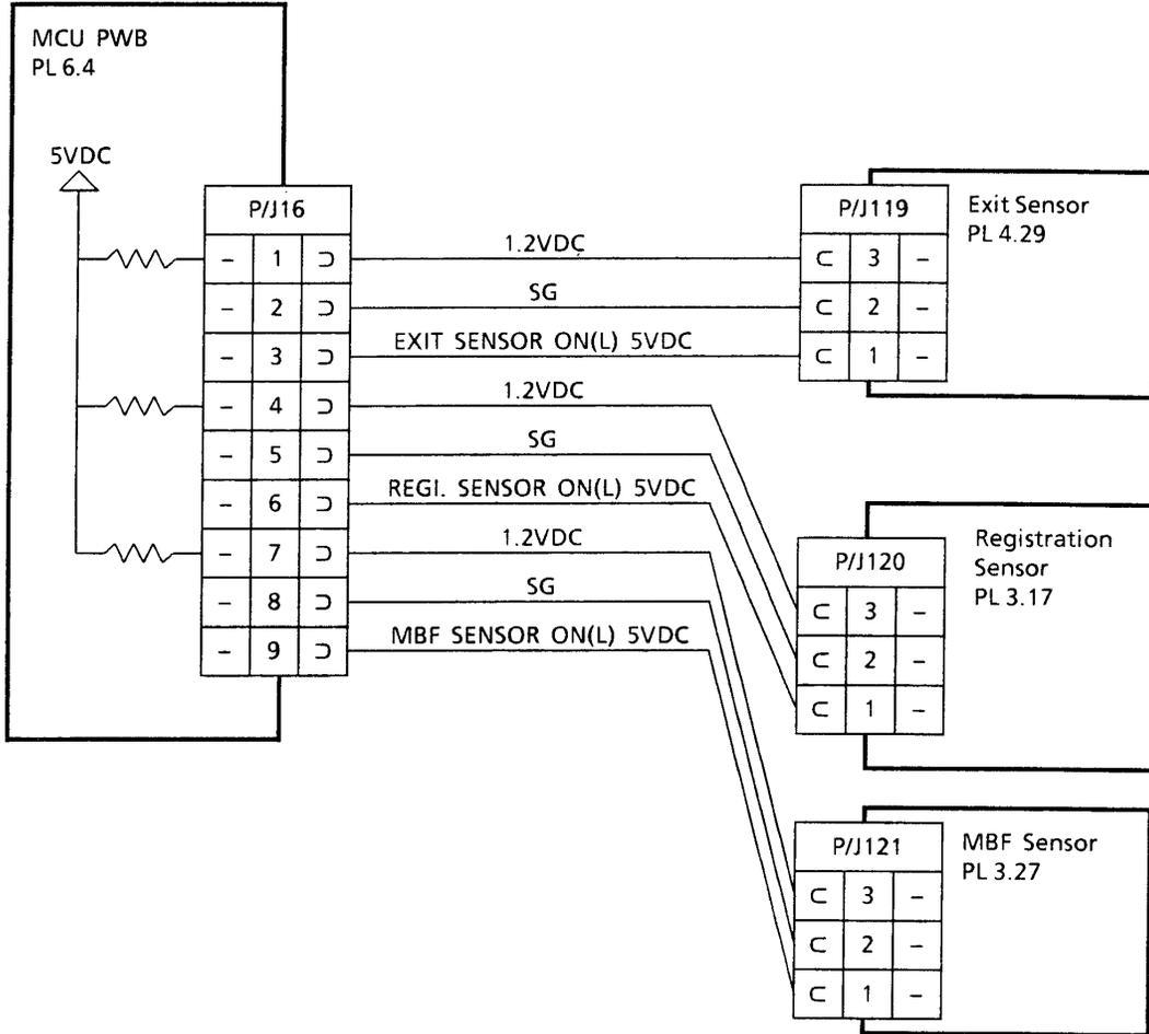
**MCU PWB, Exit Sensor, Registration Sensor, and the MBF Sensor**
