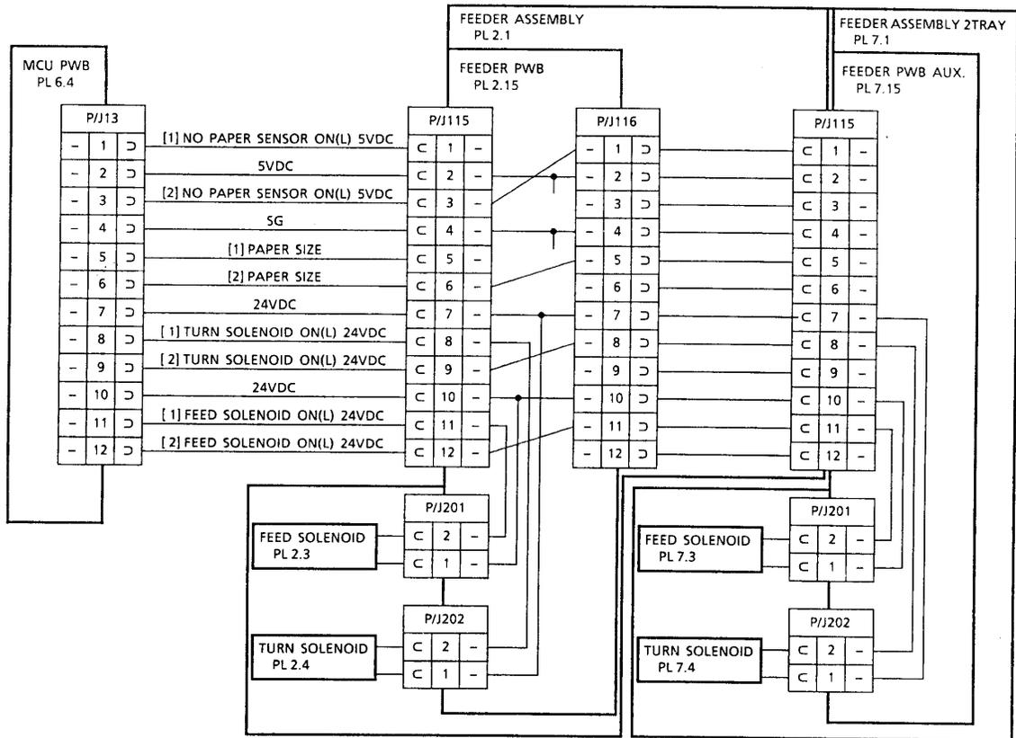
**MCU PWB, Feeder PWB, Feeder PWB AUX, Feed Solenoid, and the Turn Solenoid**
