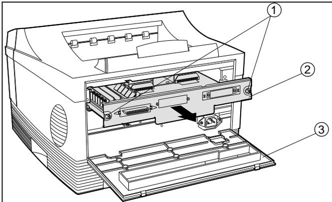
Loosen the thumbscrews and remove the system controller (ESS) board.
