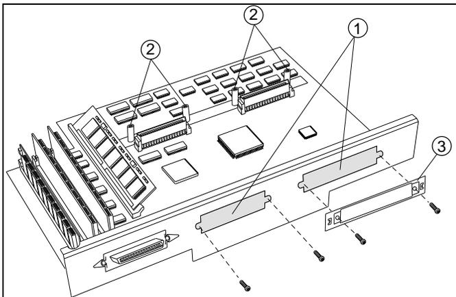
Remove the blank plate covering an interface connector slot.
