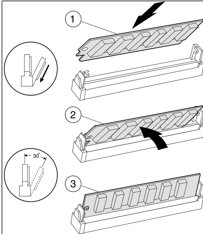
Install the option into the appropriate slot.
