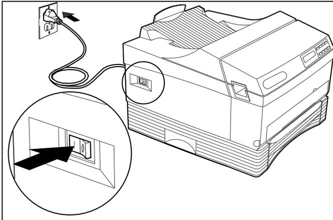
Plug in and turn on (o) the printer.
