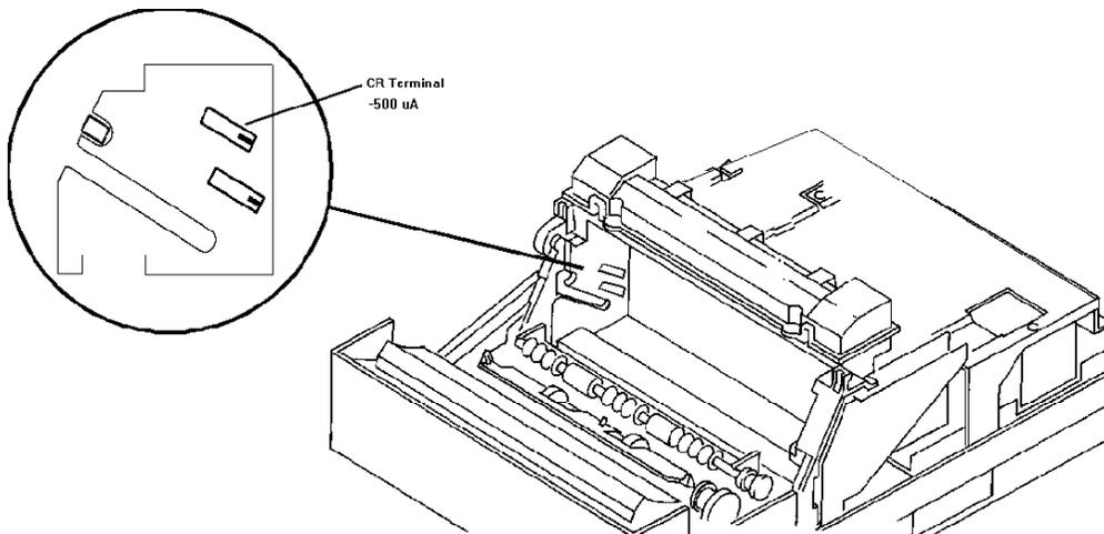
8. Use the blade of an insulated screwdriver to close the LVPS interlock switch.
