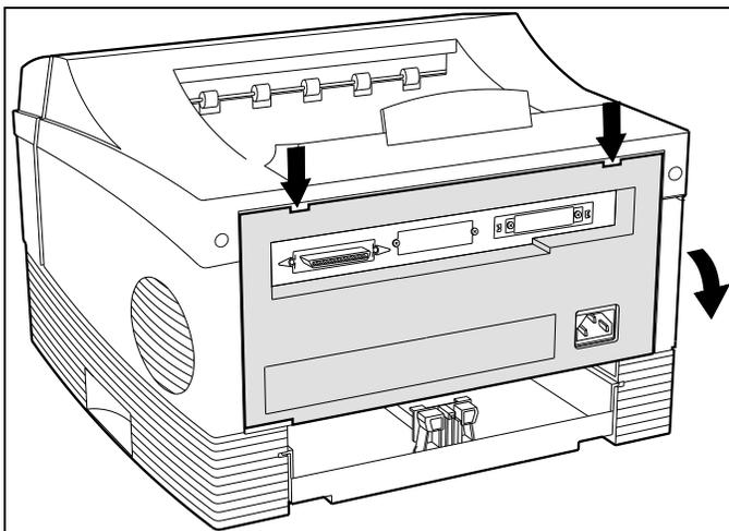
Press down on the tabs to open and lower the rear cover.
