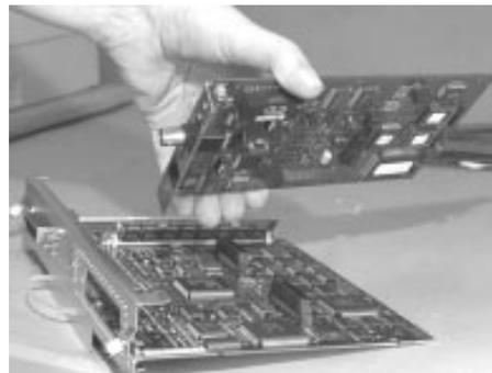
3. Align the connector on the NIC with its mate on the assembly's circuit board.
