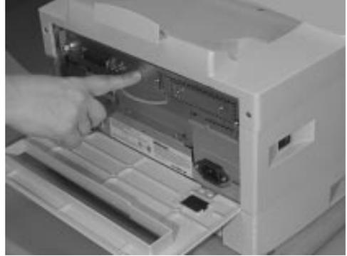
5. Unscrew the captive screws at the left and right of the assembly.
