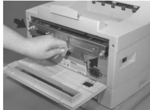
6. Pull the handle to slide the assembly from the printer. Place the assembly on a flat surface.
