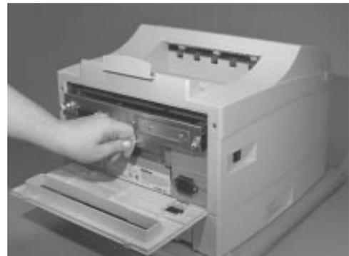
7. The NIC must be installed in the option port on the right side. Use the Phillips screwdriver to remove the plate from the option port.
