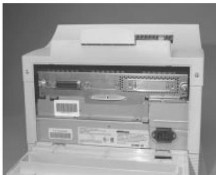
4. Touch the metal chassis to discharge static electricity.
