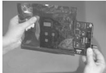
2. Insert the NIC through the option port so that its face plate is on the inside of the port.
