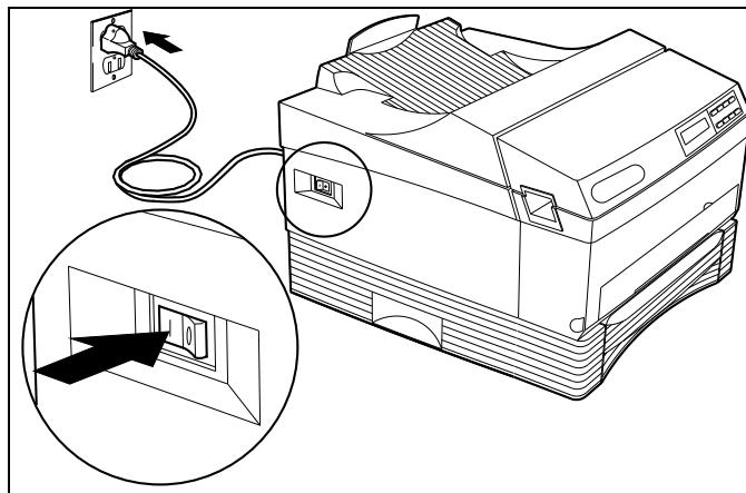
**PLUG IN AND TURN ON (I) THE PRINTER.**
