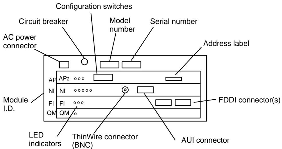
The I/O panel of the DECbridge 500/600 series units contains the following components:
