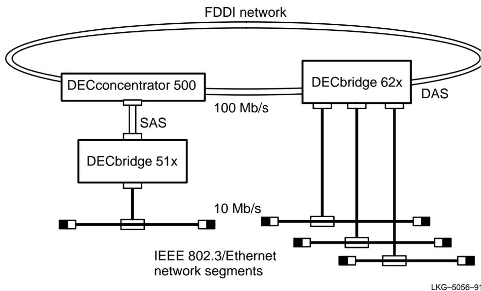
These bridges are store-and-forward devices. That is, they receive and store packets from the FDDI ring and IEEE 802.3/Ethernet network segments, then selectively filter (discard) the packets or forward them to the appropriate network.
