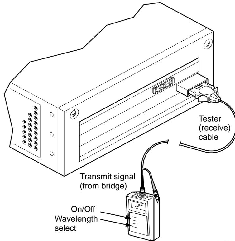
5. To measure the power of the fiber optic signal received by the bridge, refer to Figure 2-8 and follow these steps:
