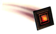
The Alpha 21264 microprocessor, with benchmarks over 30 SPECint95 and 50 SPECfp95, and with spectacular bandwidths over 4 GB/s for L2 cache and over 2 GB/s for memory, enables the system designer to produce the highest performance systems ranging from PC clients to enterprise servers. The 21264 is the third-generation 64 bit Alpha Microprocessor. It includes the latest Alpha architecture enhancements, such as motion-video instructions and byte/word operations.
