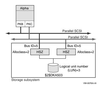
An HSZ allocation class is similar to the HSC, HSD, and HSJ allocation classes. The device name, using an HSZ allocation class number, takes the following form:
