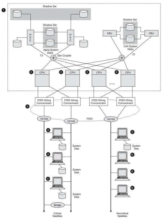
Figure 8–7 OpenVMS Cluster with Satellites
