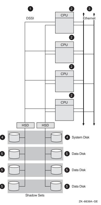
Figure 8–4 DSSI OpenVMS Cluster System
