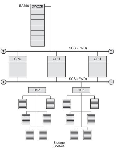
Figure 10–16 Three-Node Fast-Wide SCSI Cluster
