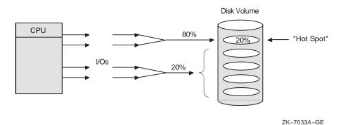
To increase the scalability of I/Os, focus on hot files, which can become a bottleneck if you do not manage them well. The activity in this area is expressed in I/Os, megabytes transferred, and queue depth.
