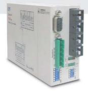
The **FIB1-SERIAL/FDC** is a asynchronous fiber optic Ring/Daisychain modem which operates over a fiber link to connect remote terminals and computers, connected in multidrop, to a central host. The **FIB1-SERIAL/FDC** allows for totally redundant, fault tolerant, self-healing operation, providing uninterrupted communications between networks nodes, even if a fiber break occurs in one or more devices in the ring or chain fails.
