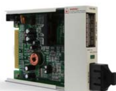
FRM301-1000MG Gigabit Multi-mode to Single mode Fiber Media Converter
