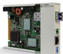
FRM301-1000TS Gigabit Ethernet 1000 Fiber Media Converter
