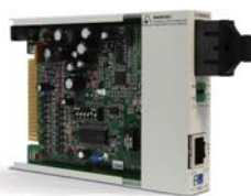
FRM301-10/100F Fast Ethernet 10/100 Fiber Media Converter
