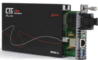
All the FRM220 series slide-in cards are available with one-slot Chassis
