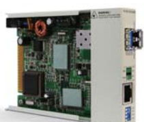
FRM301-1000ES Gigabit Ethernet 10/100/1000 Fiber Media Converter
