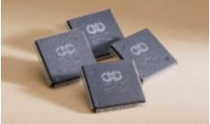
CMD's proprietary RAID chipset is the key to the CRD-5500's advanced features and incredible performance. Four separate ASICs for RAID (Exclusive OR), cache control, CPU-I/O (CPU support logic), and DMA (high speed internal data bus) functions support the industry's most advanced architecture.
