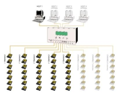
CMD provides almost unlimited configuration options! Up to nine SCSI modules can be installed for host (up to four) or disk (up to eight) use, supporting up to 120 disk drives and 32 logical devices (LUNs). RAID sets may be configured in any orientation and freely moved within the CRD-5500's SCSI disk channels.
