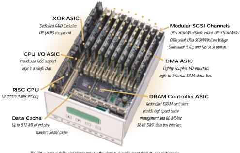
The CRD-5500's scalable architecture provides the ultimate in configuration flexibility and performance, allowing you to easily upgrade or enhance the capabilities of your RAID peripheral investment!
