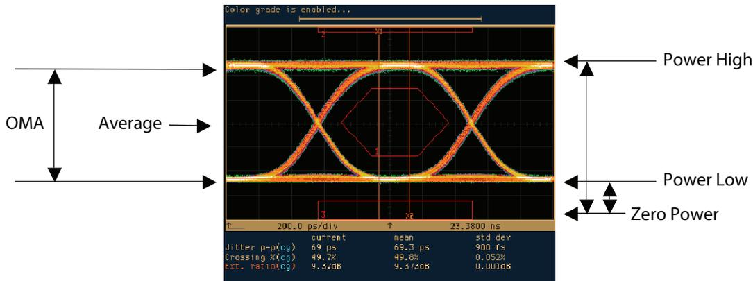
Figure 6. Eye diagram illustrating optical figures of merit: average power, OMA, power high, power low and zero level power.
