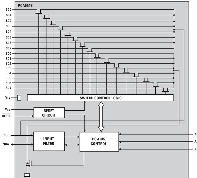
Figure 5. Example block diagram of a two-wire serial bus switch (from Philips "PCA9548 8-channel I<sup>2</sup>C switch with reset" IC datasheet).
