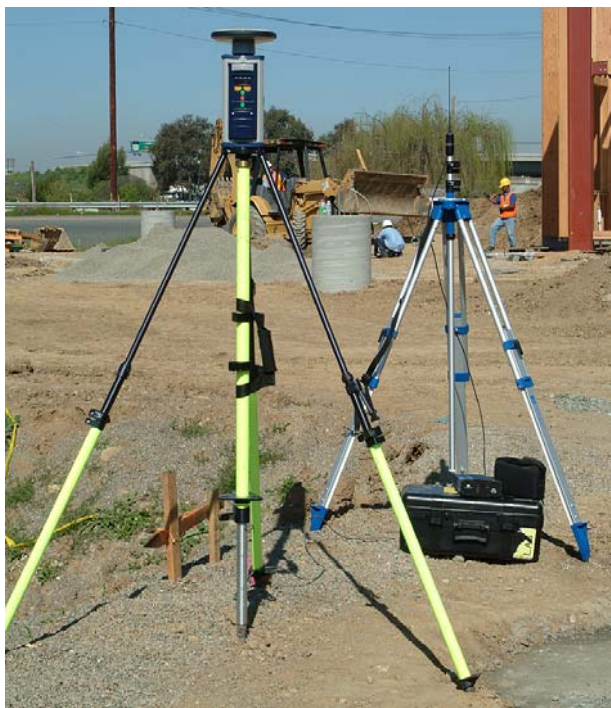
Figure 11 RTK Base Setup with Pacific Crest PDL Radio
