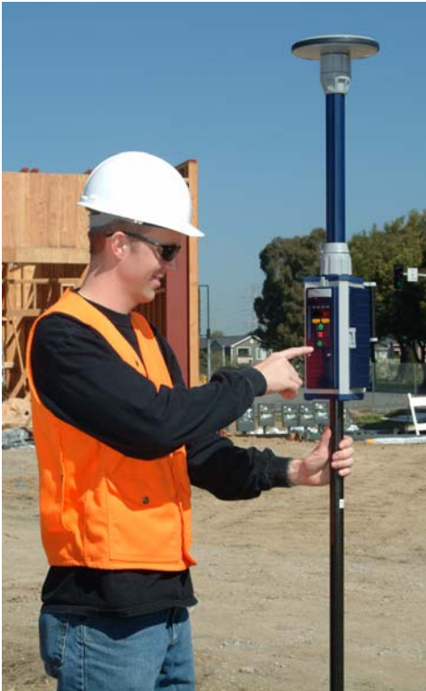
Figure 12 Pole-Mounted RTK Rover Setup
