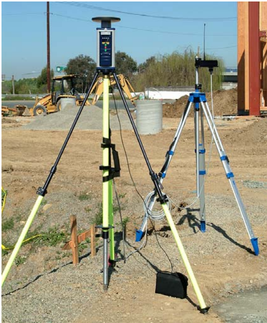
Figure 10 RTK Base Setup with Thales U-Link Radio
