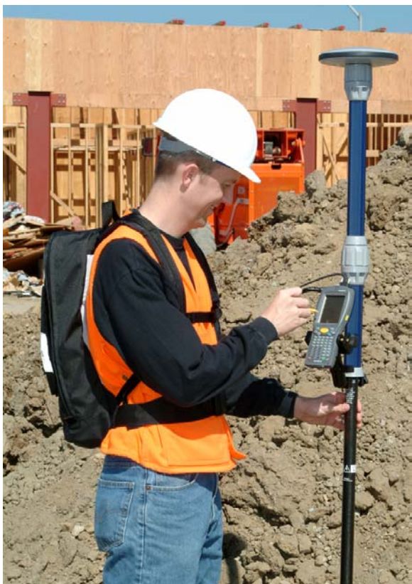
Figure 13 Backpack-Mounted RTK Rover Setup
