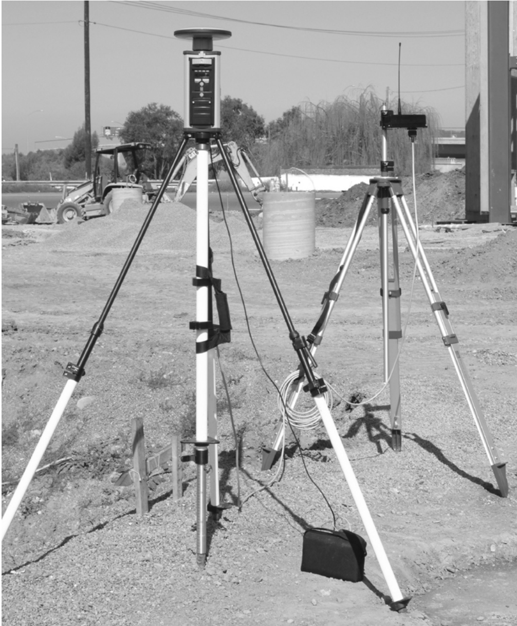
Figure 10 RTK Base Setup with Thales U-Link Radio
