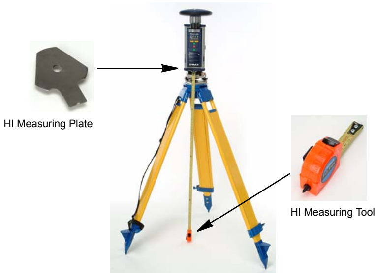
Figure 4.4 Measuring HI (Height of Instrument) of Base GPS Antenna
