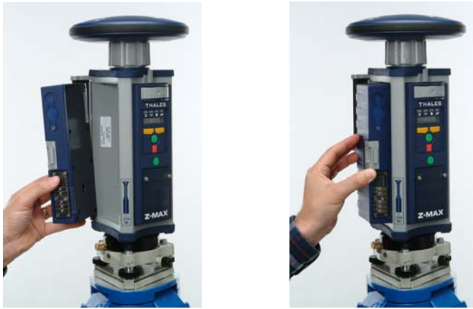
Figure 3.2 Connecting Power Module to GPS Receiver Module
