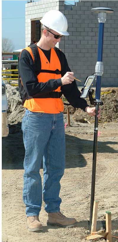
Figure 3.24 Fully Connected Pole-Mounted Rover System
