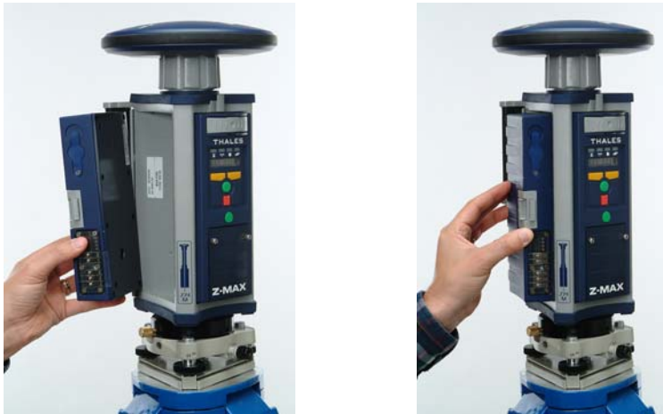
Figure 2.10 Connecting the Power Module to the GPS Receiver Module
