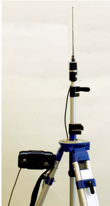
Figure 4.3 Mounted PDL Base Radio Antenna
