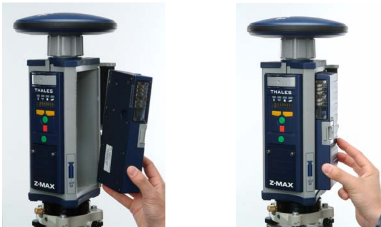
Figure 3.25 Connecting Communication Module to GPS Receiver Module
