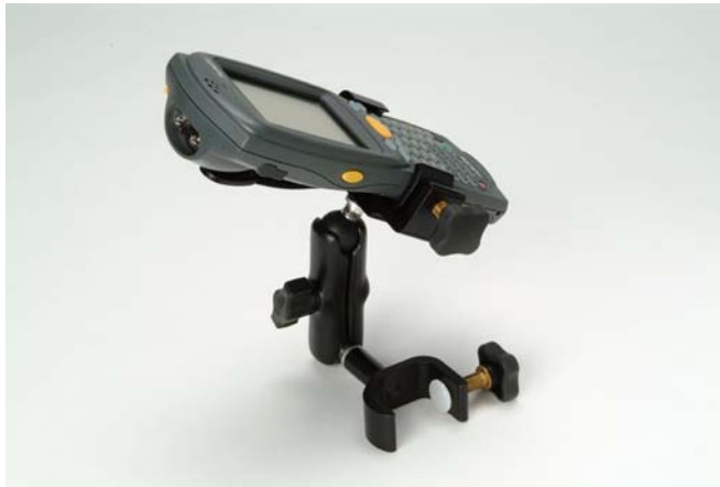
Figure 4.8 FAST Terminal Handheld Computer Mounted on Rover Pole
