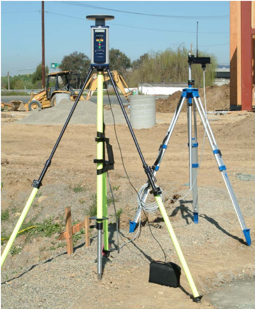
Figure 3.13 Connecting Thales U-Link Radio & Z-Max GPS Receiver Module
