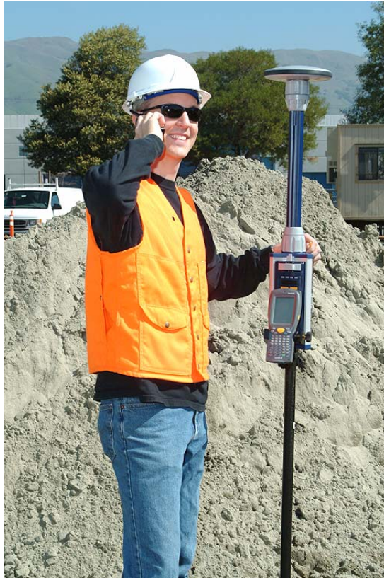
Figure 4.7 Pole-Mounted Rover System Ready to Survey
