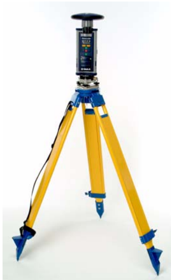
Figure 3.7 GPS Receiver Module Adjustable Tripod Installation
