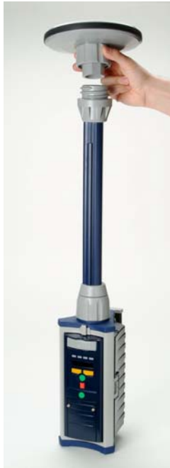
Figure 3.20 GPS Antenna Module - UHF Antenna Module Connection
