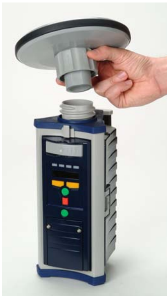
Figure 3.4 Connecting GPS Antenna Module to GPS Receiver Module
