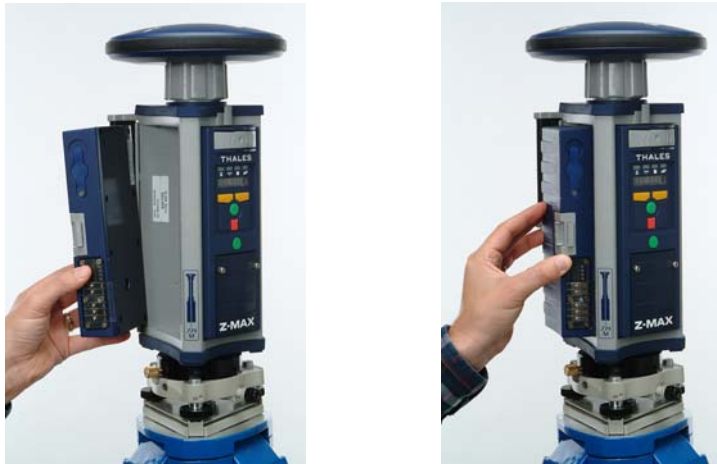
Figure 3.2 Connecting Power Module to GPS Receiver Module
