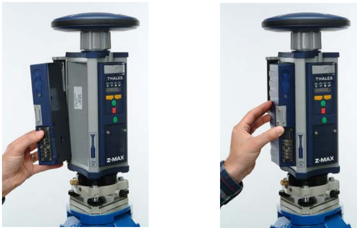
Figure 3.1 GPS Receiver - Power Module Connection
