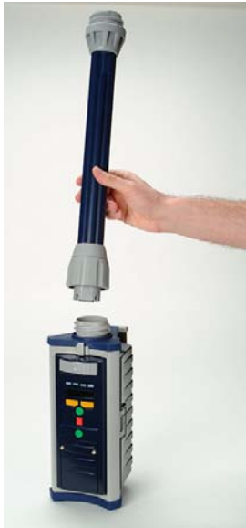
Figure 3.19 UHF Antenna Connection to GPS Receiver Module
