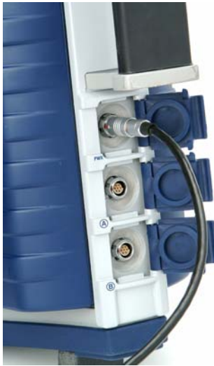
Figure 3.2 External Power Connection
