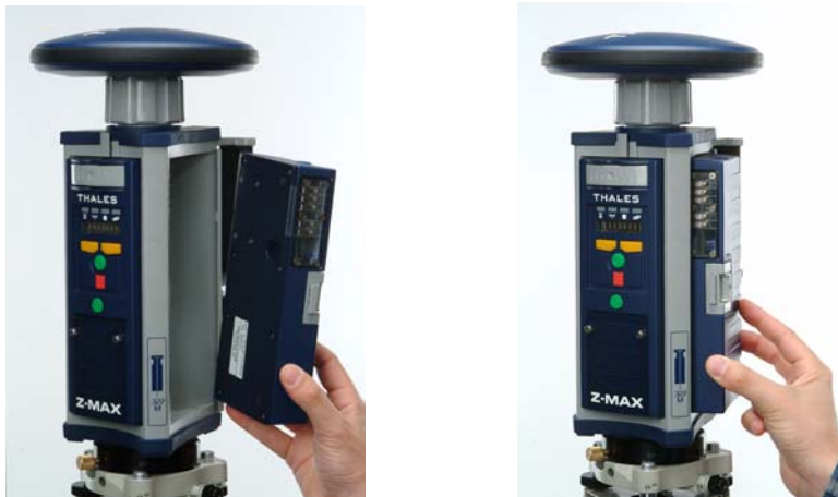
Figure 2.13 Connecting Communication Module to GPS Receiver Module
