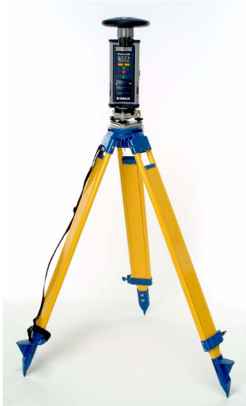
Figure 4.5 Z-Max Survey System Performing a Static Survey
