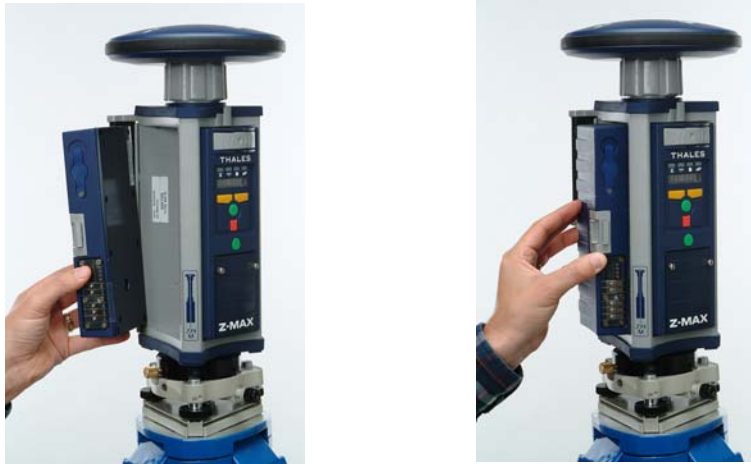
Figure 3.26 GPS Receiver - Power Module Connection
