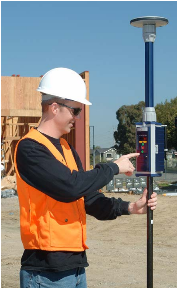
Figure 4.6 Pole-Mounted Rover System
