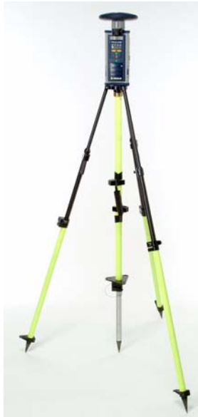
Figure 3.6 GPS Receiver Module Fixed Height Tripod Installation
