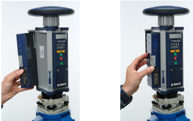
Figure 3.22 GPS Receiver - Power Module Connection
