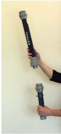
Figure 3.30 UHF Antenna/Range Pole RF Adapter Connection
