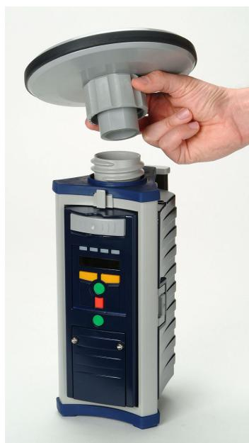
Figure 4 Connecting GPS Antenna Module
