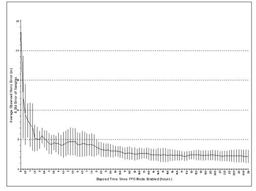
Figure 4.11: Point Positioning Mode Position Error - GPS Only
