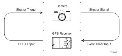
Figure 4.9: Closed Loop Technique
