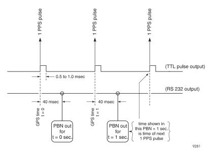
Figure 4.6: Relationship of GPS Time in PBN Record to 1 PPS Pulse
