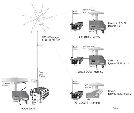
Figure 5.1: Combined Differential/RTK Base Station and Remote Operation
