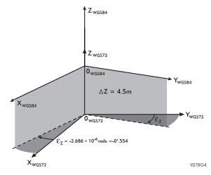
Figure 6.2: Rotation and Translation Between Coordinate Systems
