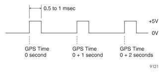
Figure 4.7: 1PPS Characteristics
