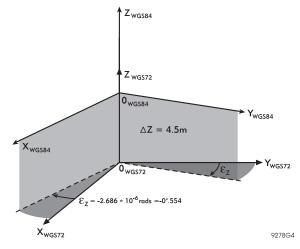
Figure 4.10: Rotation and Translation Between Coordinate Systems
