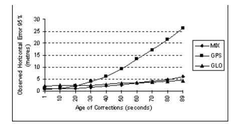
Figure A.1: GG Surveyor Code Differential Horizontal Position Decay
