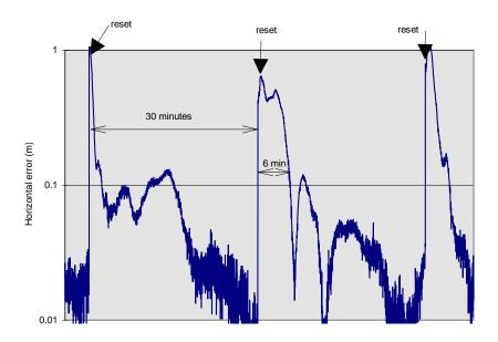
Figure 5.3: Convergence of Float Solution Following Reset
