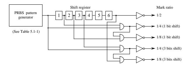
Fig. 5.1-1 Mark Ratio 1/4, 1/8 Pattern Generator
