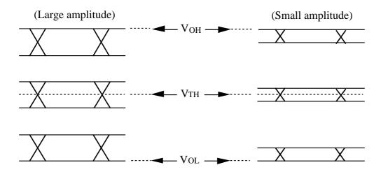
Fig. 4.3.5-1 Offset Reference Value and Amplitude Change
