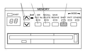
Insert the floppy disk into the floppy disk drive and select the file name to be deleted.
