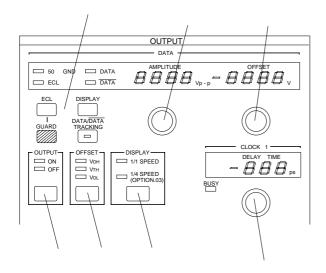
When you want to set front panel DATA/DATA output and CLOCK 1/CLOCK 1 output, switch to 1/1 SPEED. When you want to set rear panel 1/4 SPEED OUTPUT (OPTION), switch to 1/4 SPEED.
