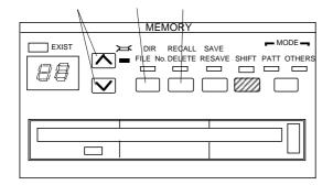
Insert the floppy disk into the floppy disk drive and select the DIR mode. If the floppy disk is changed, always execute a DIR command.
