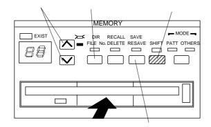
Insert a formatted floppy disk (2HD, 2DD) into the floppy disk drive. (For a description of how to format a floppy disk, see section 4.4.3 "Disk formatting".)
