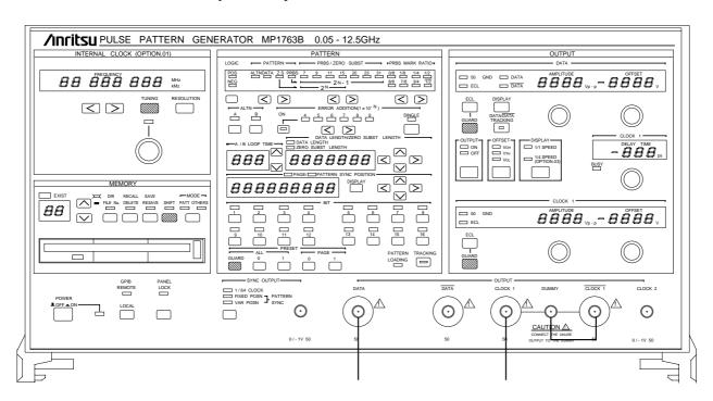
Fig. 6.3-1 Connection of front panel
