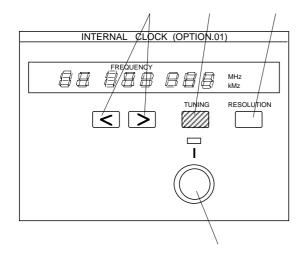
Press the TUNING key. The TUNING lamp lights. (The frequency can be changed only when the TUNING lamp is lit.) At this time, the figure of the digit that can currently be changed blinks.
