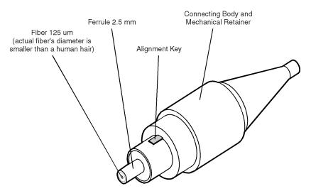
Figure 3-1. Basic components of a connector.
