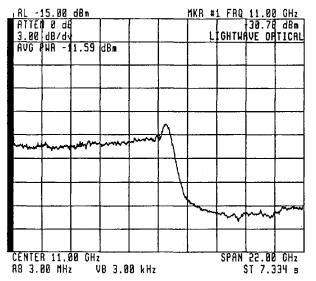
Figure 4-4. Chirp Under Sinusoidal Modulation (Modulation frequency = 100 MHz)
