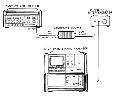
Figure 5-2. Interferometric Test Setup
