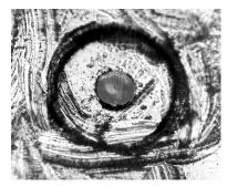
Figure 3-6. Damage from improper cleaning.
