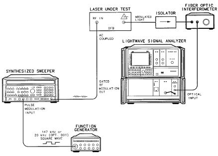
Figure 4-3. Typical Modulated Laser Power Spectrum Test Setup for Chirp Measurement
