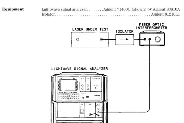
Figure 4-1. Static Linewidth Measurement Test Setup
