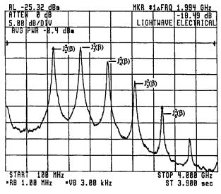
Figure 4-5. FM Sidebands Shown by Low-Level Chirp (Modulation frequency = 500 MHz)
