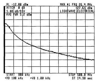
Figure 4-2. DFB Linewidth Measurement with Agilent 71400C
