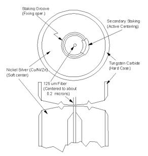
Figure 3-3. Cross-section of the Diamond HMS-10 connector.
