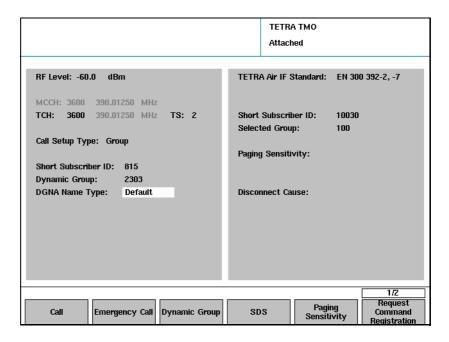
6 Set up the call parameters as explained in "Setting up the call parameters" on page 44. In particular, enter the call setup type and Short Subscriber ID; the dynamic group number is not required in an individual call.
