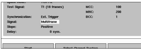
In this field, you should indicate if the trigger signal occurs at the beginning of every new downlink frame (ie. every 56.67 ms) or every multiframe (1.02 s).
