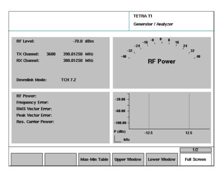
4 Select a signal type in the Downlink Mode field: TCH 7.2 (the Stabilock transmits four time slots per frame, one containing a typical TCH/7.2 signal, the other slots filled with dummy bursts)
