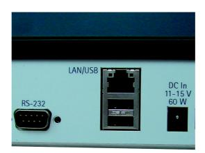
In addition to operating the 2305 Stabilock through its front panel elements, it can also be controlled remotely from a PC through the serial (RS-232) interface or the LAN (local area network).
