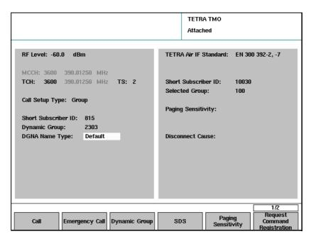
6 Set up the call parameters as explained in "Setting up the call parameters" on page 44. In particular, enter the call setup type (Individual Duplex or Individual Simplex); the Short Subscriber ID and the dynamic group number are not required in an individual, outgoing call.
