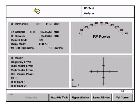
Once the 2305 Stabilock is synchronized with the base station, the synchronization symbol in the top-left corner changes, and the transmitter measurements are started.
