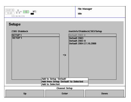
5 Push Add to Setup 'Default' if you want to copy the channel setups from the selected setup file to the Default setup file on the Stabilock. Or: Push Add from Setup 'Default' to Selected if you want to copy the channel setups from the Default setup file on the Stabilock to the selected setup file.
