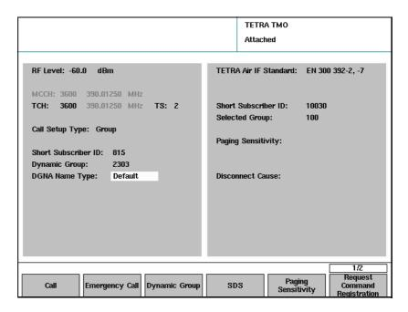
6 Set up the call parameters as explained in "Setting up the call parameters" on page 44. In particular, enter the call setup type and the dynamic group number; the Short Subscriber ID is not required in an incoming group call.
