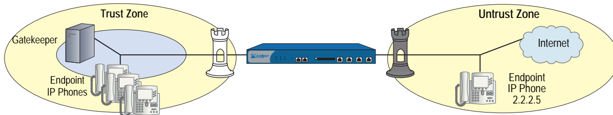
Figure 2: H.323 Gatekeeper in the Trust Zone
