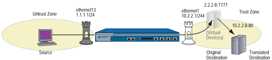
Figure 10: NAT-Dst with Port Mapping
