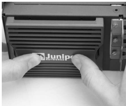
Figure 25: Securing Filter Cover
