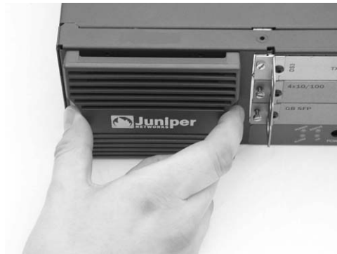
Figure 22: Squeezing Filter Cover Tabs
