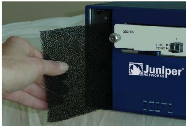
7. Carefully insert a new filter into the chassis. Use the wooden ruler as an aid to guide the back edge of the filter to the end of the Velcro wall.
