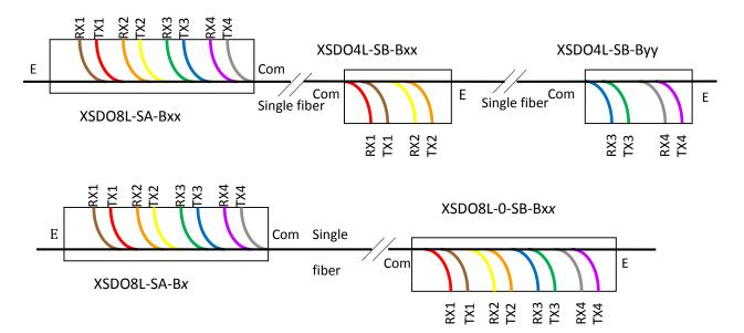
Figure 1 Multichannel single fiber connection examples
