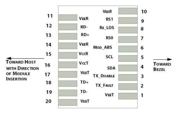
Figure 1: Interface to Host PCB
