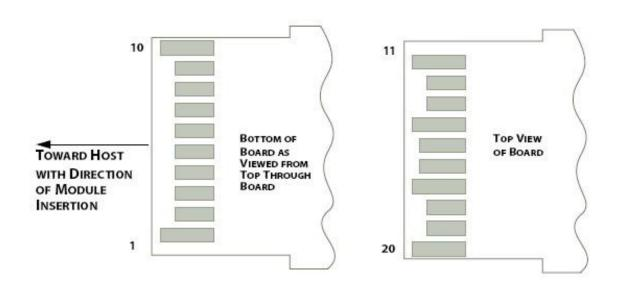
Figure 2: Module Contact Assignment
