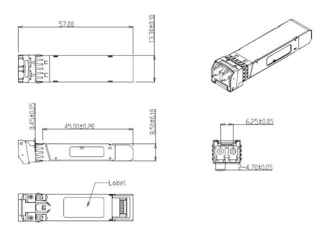
Figure 5. Mechanical Specifications
