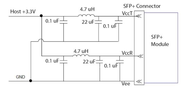
Figure 3. Host Board Power Supply Filters Circuit
