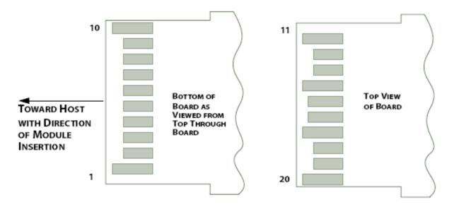
Figure 2: Module Contact Assignment
