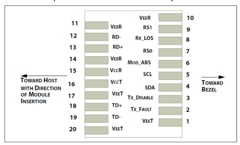
Figure 3: Module Interface to Host
