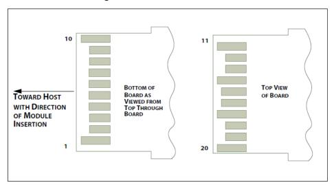
**Figure 4: Module Contact Assignment**
