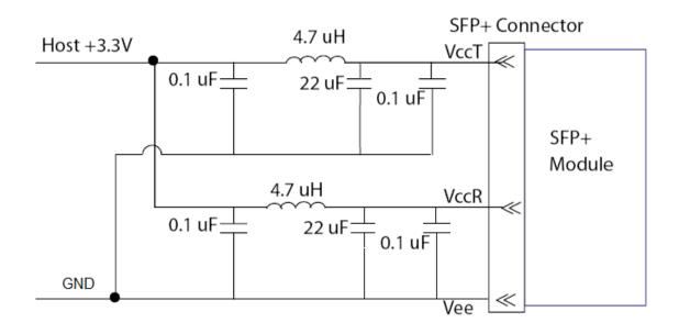
Figure 3. Host Board Power Supply Filters Circuit
