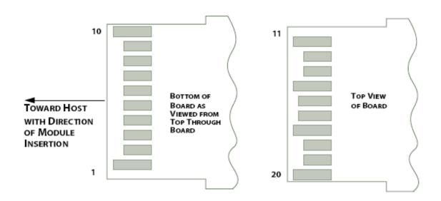
**Figure 2: Module Contact Assignment**
