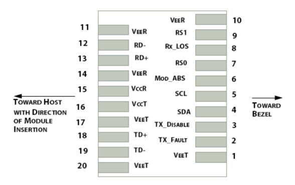
Figure 1: Interface to Host PCB
