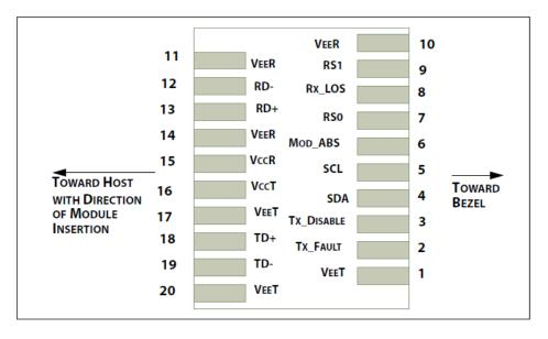
Figure 3: Module Interface to Host
