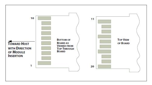
Figure 4: Module Contact
