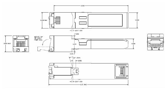
Figure 2. XSUEx1-M1RN mechanical dimensions
