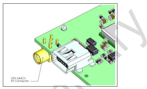
Figure 5: MMCX connector for antenna connection
