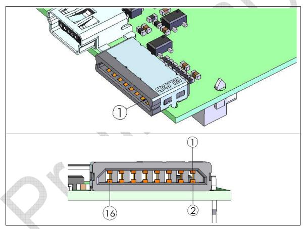
Figure 7: 16-Way IO Expander Socket
