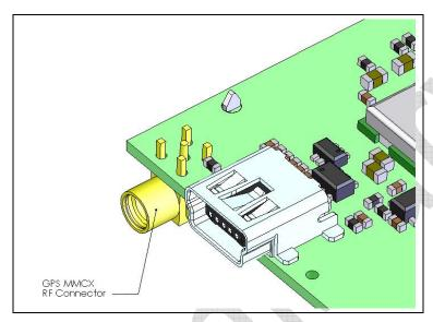
Figure 5: MMCX connector for antenna connection
