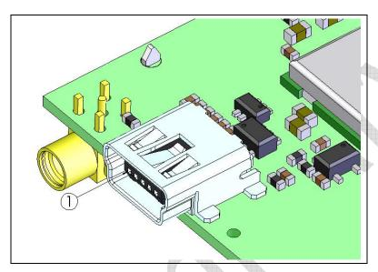
Figure 6: Mini-B USB connector
