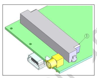
Figure 7: IESM 50-pin connector
