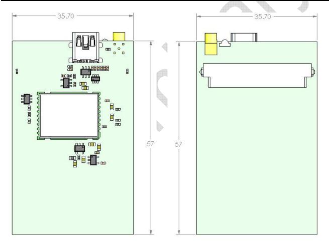
Figure 8: IESM-GPS+USB Dimensions
