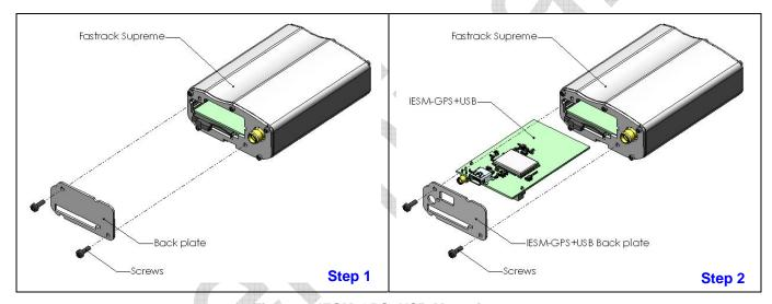
Figure 9: IESM-GPS+USB Mounting
