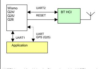
UART2 is used for driving the Bluetooth module. UART2 carry the commands compatible with HCI protocol. The type of UART2 is 4 wires with flow control. Speed\* and format can be tuned to adapt with BT Chipset type. \*Up to 115.2kbps
