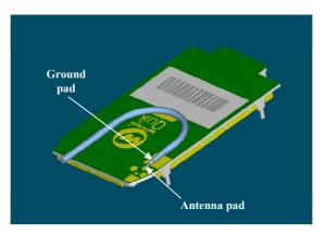
Figure 7: Antenna connection
