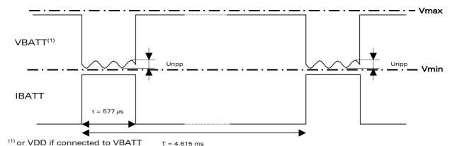
Figure 2: Typical power supply voltage in GSM mode
