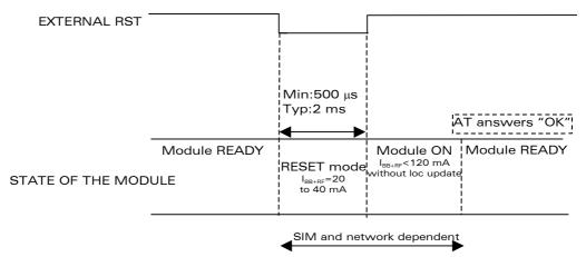
Figure 6: Reset sequence diagram
