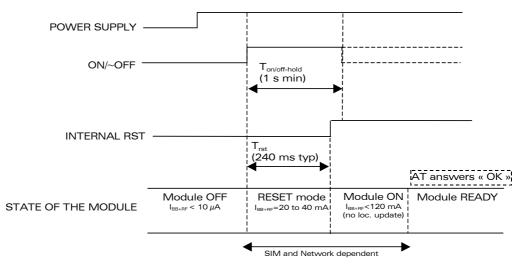
$I_{BB+RF}$  = overall current consumption (Base Band + RF part)
