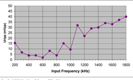
for f<100kHz U<sub>ripp</sub> Max = 50mVpp for f> 1800kHz U<sub>ripp</sub> Max = 40 mVpp
