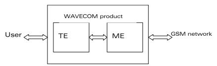
A call from a GSM mobile station to the PSTN is called a "mobile originated call" (MOC) or "outgoing call", and a call from a fixed network to a GSM mobile station is called a "mobile terminated call" (MTC) or "incoming call".
