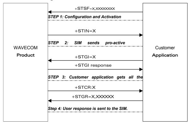
On the first step, the customer application informs the WAVECOM product which facilities are supported. This operation is performed with the **+STSF** (SIM ToolKit Set Facilities) command, which also allows to activate or deactivate the SIM Toolkit functionality.
