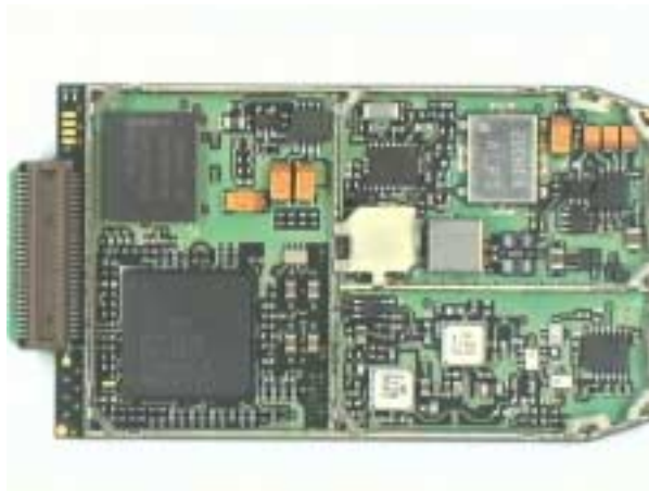
Figure 1 : WISMO2C2 and WISMO2C2-RFC (bottom view)
