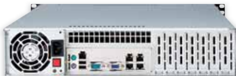
Rear View (Fits any standard I/O shield)
