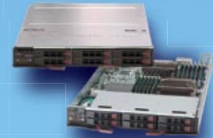
2-way Intel Processor Blade w/ Six 2.5" Hot-plug Drive Bays
