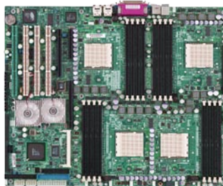
H8QC8/H8QCE H8QC8+*/H8QCE+* *(+)versions are optimized for 1U chassis with PCI-X slots removed
