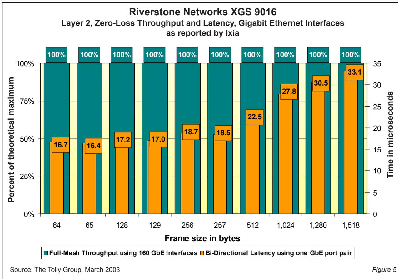
Tolly Group engineers connected each device under test to an IXIA 1600T traffic generator/analyzer using 1310nm single mode fiber with the 10-Gigabit Ethernet interfaces and 62.5micron multimode fiber with the Gigabit Ethernet interfaces. (See Figure 5.)
