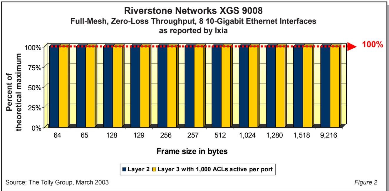
both switches in port-pairing and full-mesh configurations at Layer 2 and Layer 3, and at Layer 3 with access control lists (ACLs) active on the 10-Gigabit Ethernet interfaces. Engineers also conducted tests with Gigabit Ethernet interfaces at Layer 2 only. (Note: Jitter was not reported in a full-mesh configuration.) 10-Gigabit
